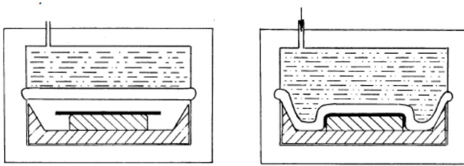
Figure 1.6: Fluid cell rubber forming [45]
