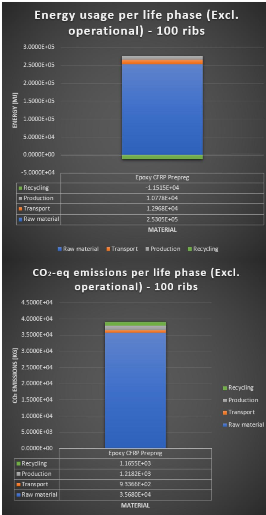
Figure 3.9: Epoxy CFRP prepreg energy and CO<sub>2</sub> per life stage charts (excluding the operational phase)
