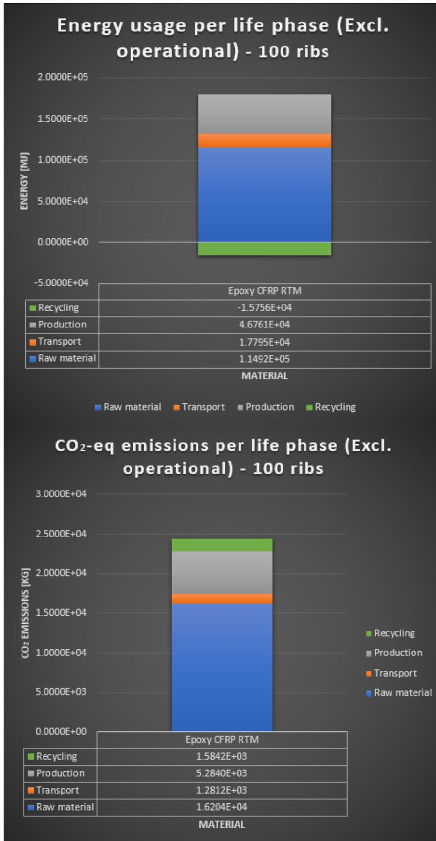
Figure 3.12: Epoxy CFRP RTM energy and CO<sub>2</sub> per life stage charts (excluding the operational phase)
