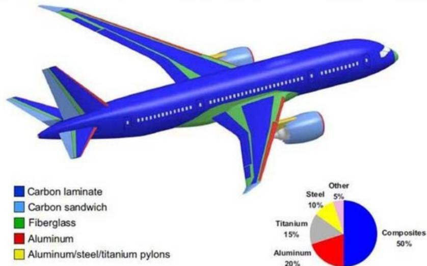
Figure 1.3: Materials used in a Boeing 787 [32]
