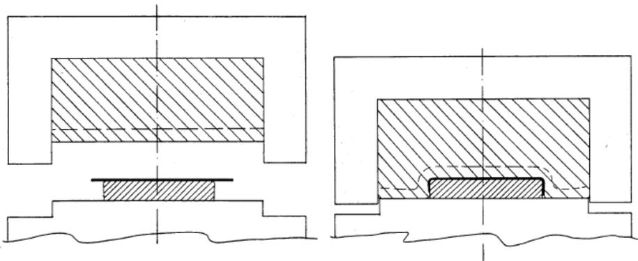
Figure 1.7: Solid rubber pad forming [45]
