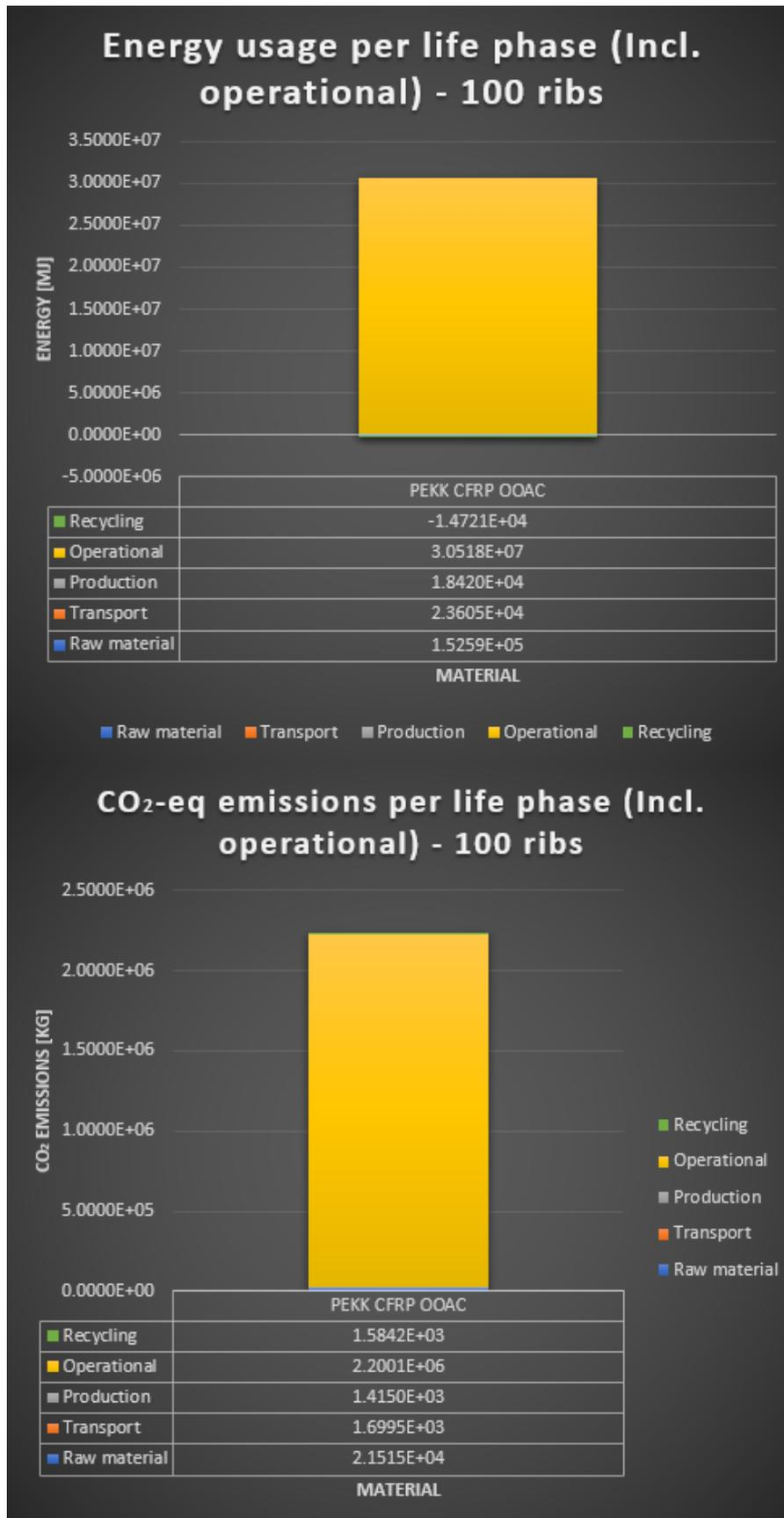
**Figure 3.16:** PEKK CFRP OOAC (hot press consolidation) energy and CO<sub>2</sub> per life stage charts (including the operational phase)
