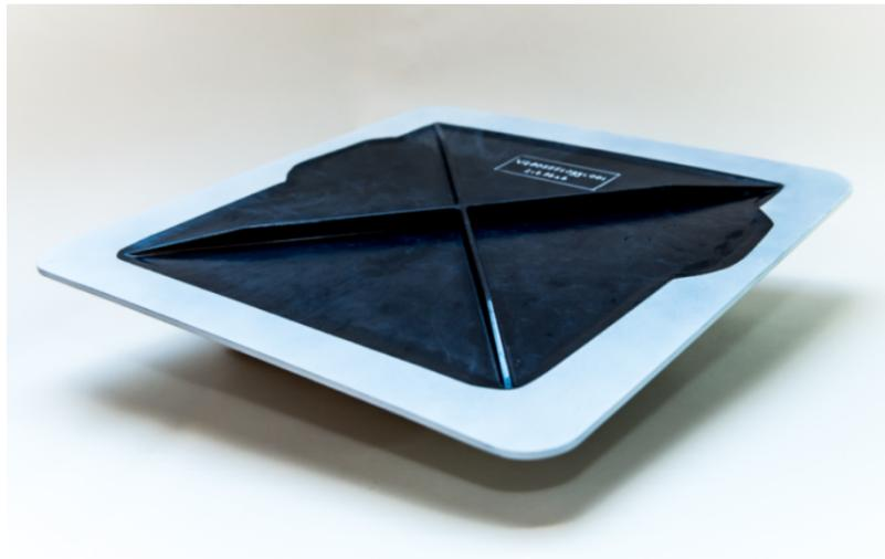
**Figure 2.6:** Bell v280 Valor, rotorcraft access panel. Photo credits: GKN Fokker [56]
