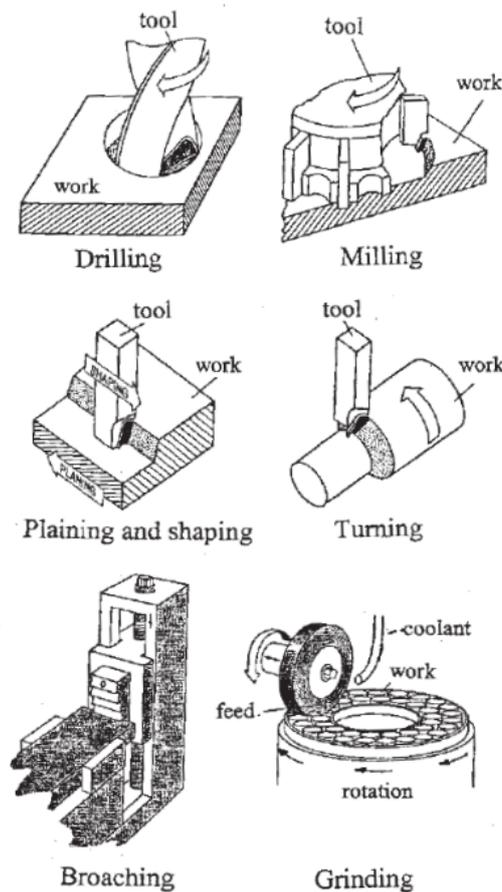
Figure 1.4: Machining processes [31]
