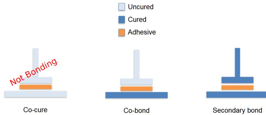
Figure 1.10: Co-curing (co-consolidation), co-bonding and secondary bonding of composites [12]
