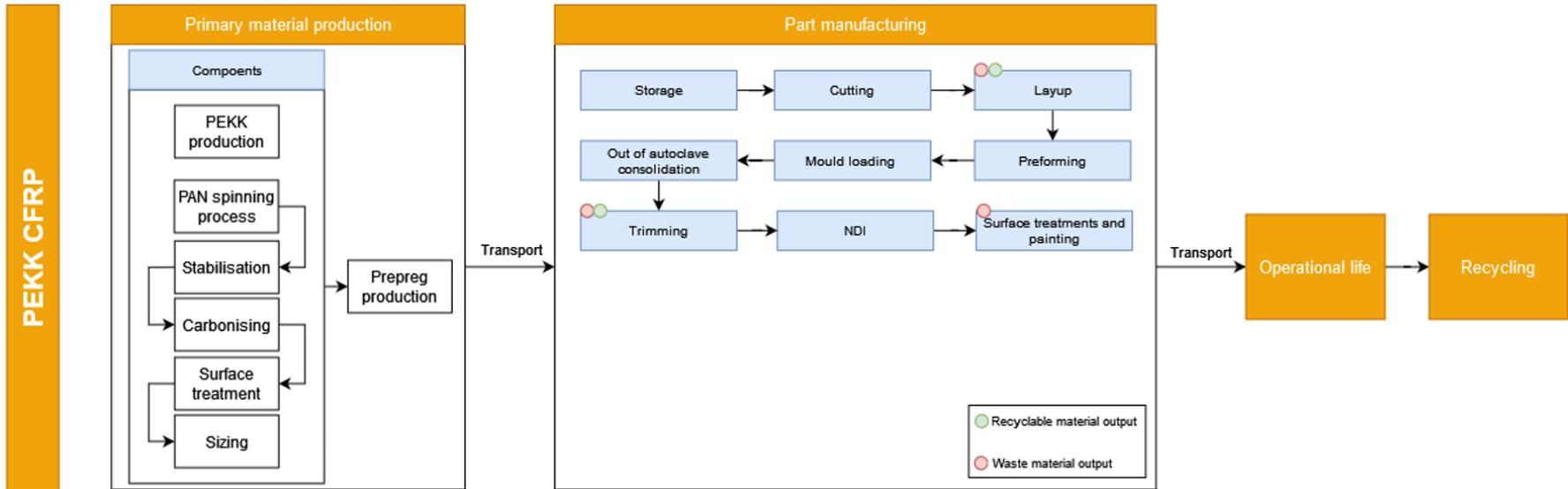
Figure 2.4: Thermoplastic process flow chart
