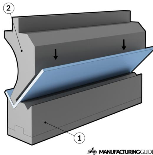
Figure 1.5: Press brake bending process [36]
