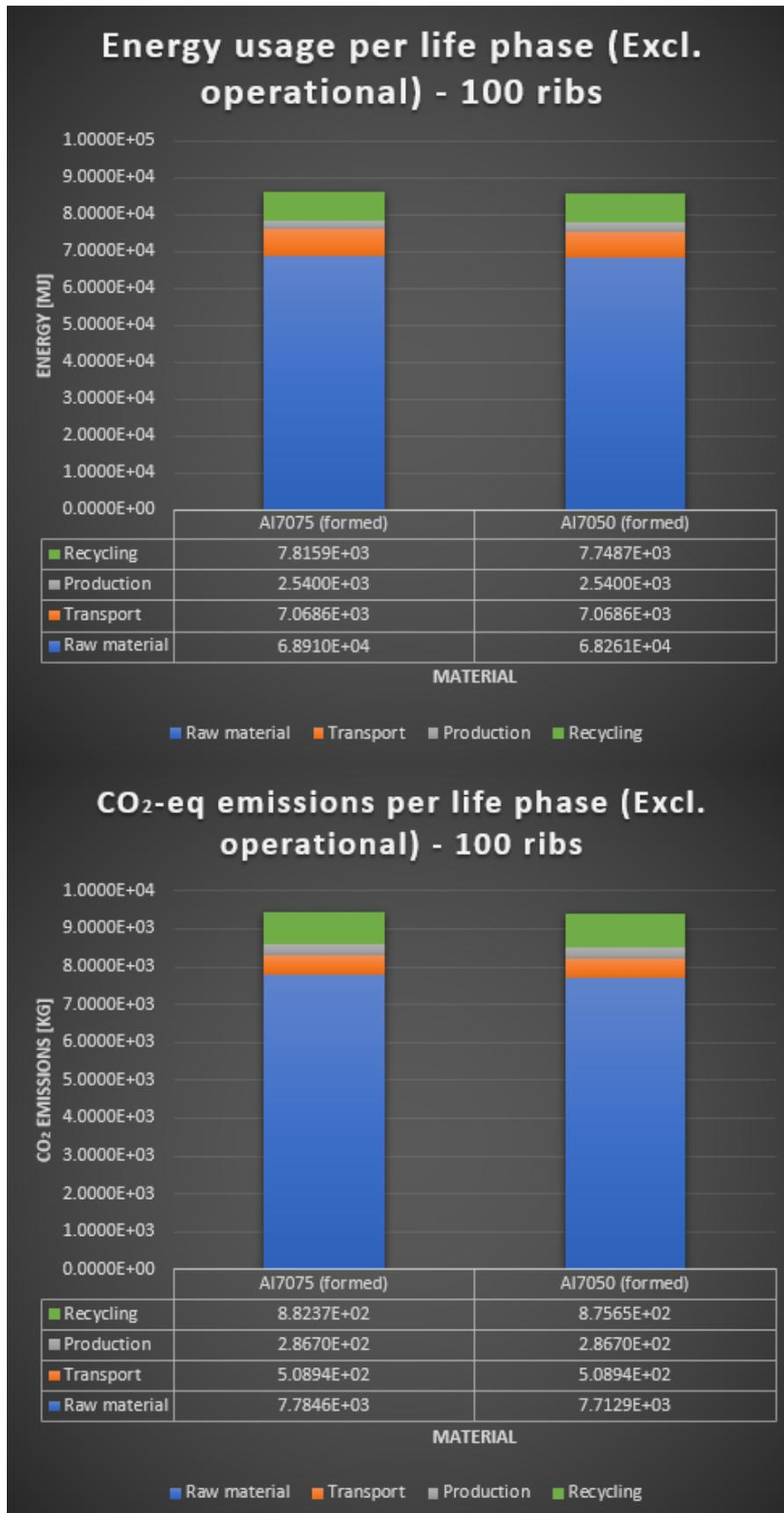
Figure 3.6: Sheet formed aluminium energy and CO<sub>2</sub> per life stage charts (excluding the operational phase)
