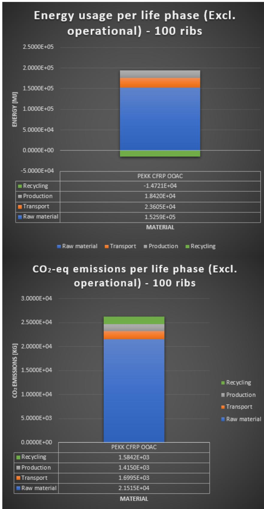
**Figure 3.15:** PEKK CFRP OOAC (hot press consolidation) energy and CO<sub>2</sub> per life stage charts (excluding the operational phase)
