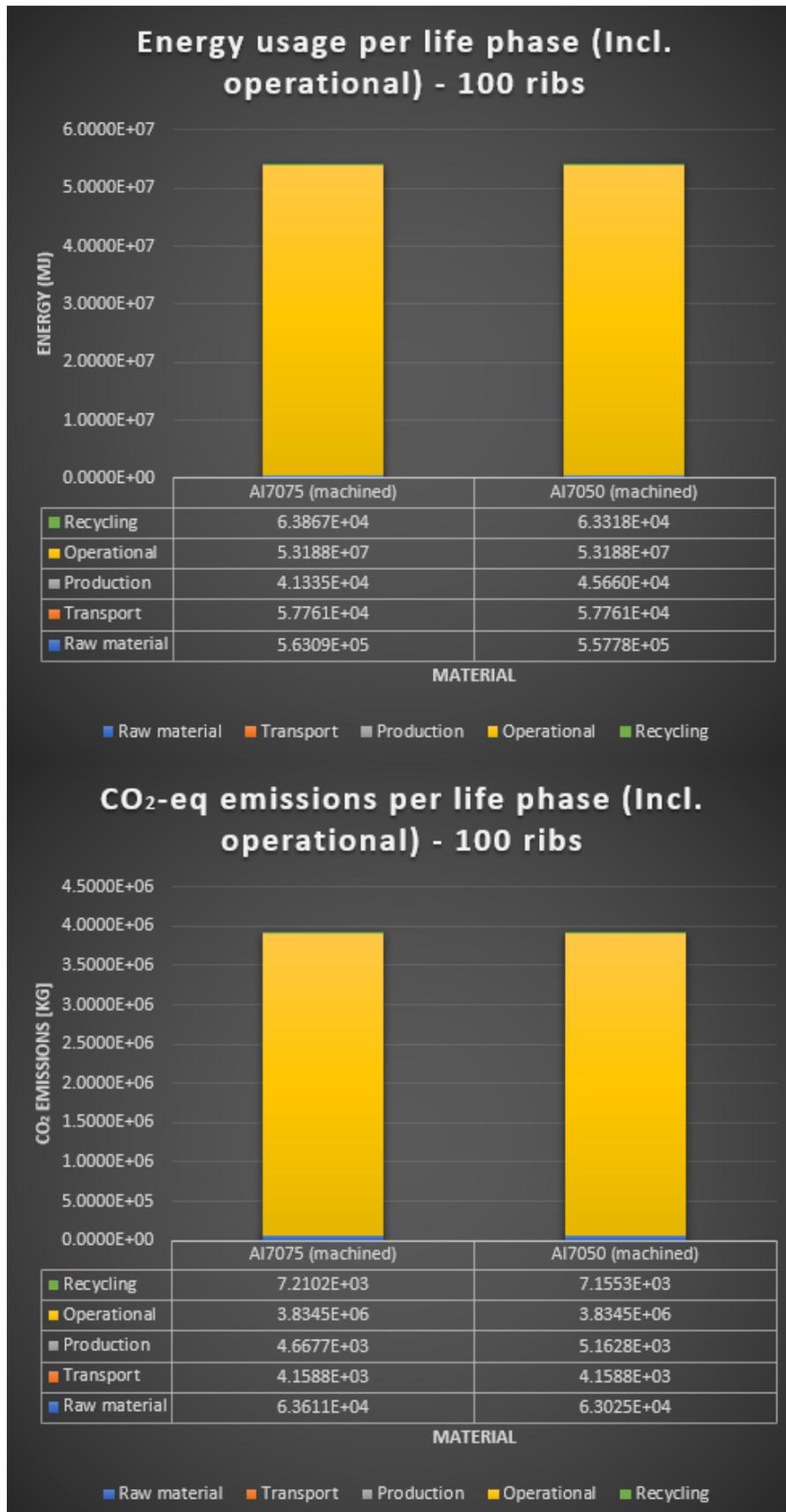
Figure 3.4: Machined aluminium energy and CO<sub>2</sub> per life stage charts (including the operational phase)
