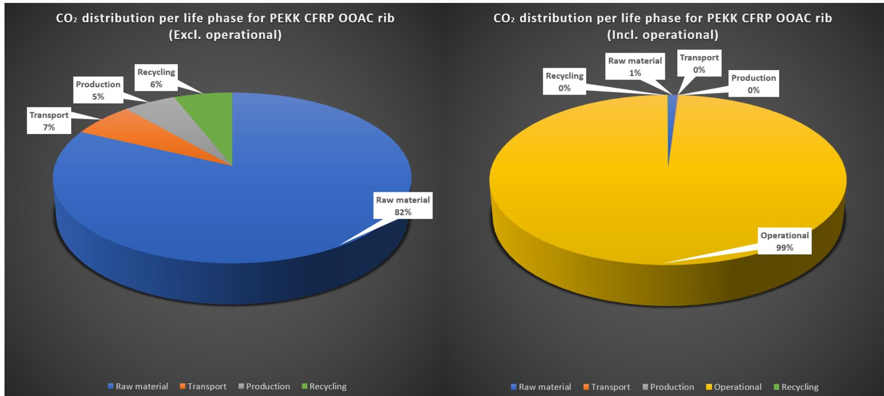
**Figure 4.9:** CO<sub>2</sub>-eq distribution per life phase for PEKK CFRP OOAC rib
