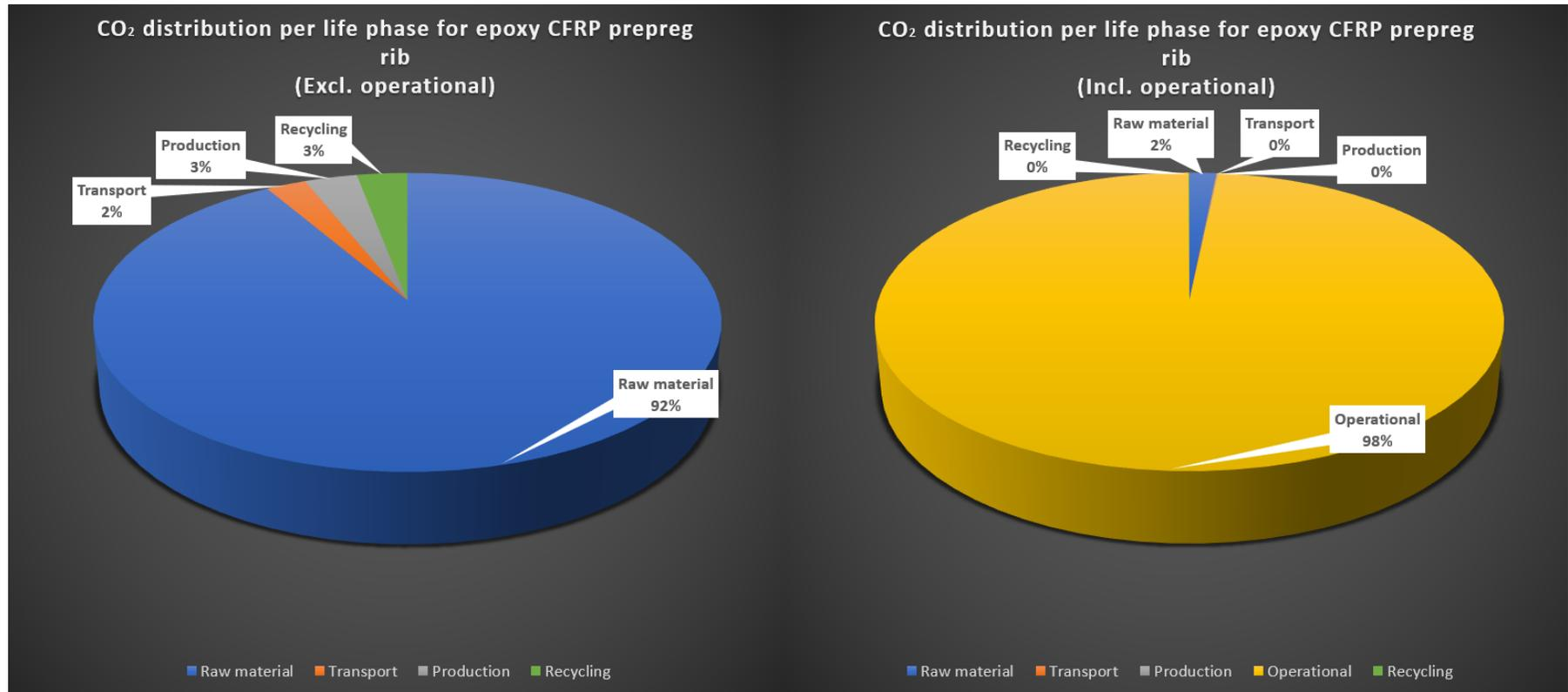
**Figure 4.7:** CO<sub>2</sub>-eq distribution per life phase for epoxy CFRP prepreg rib
