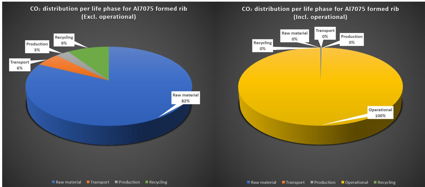
**Figure 4.6:** CO<sub>2</sub>-eq distribution per life phase for Al7075 formed rib
