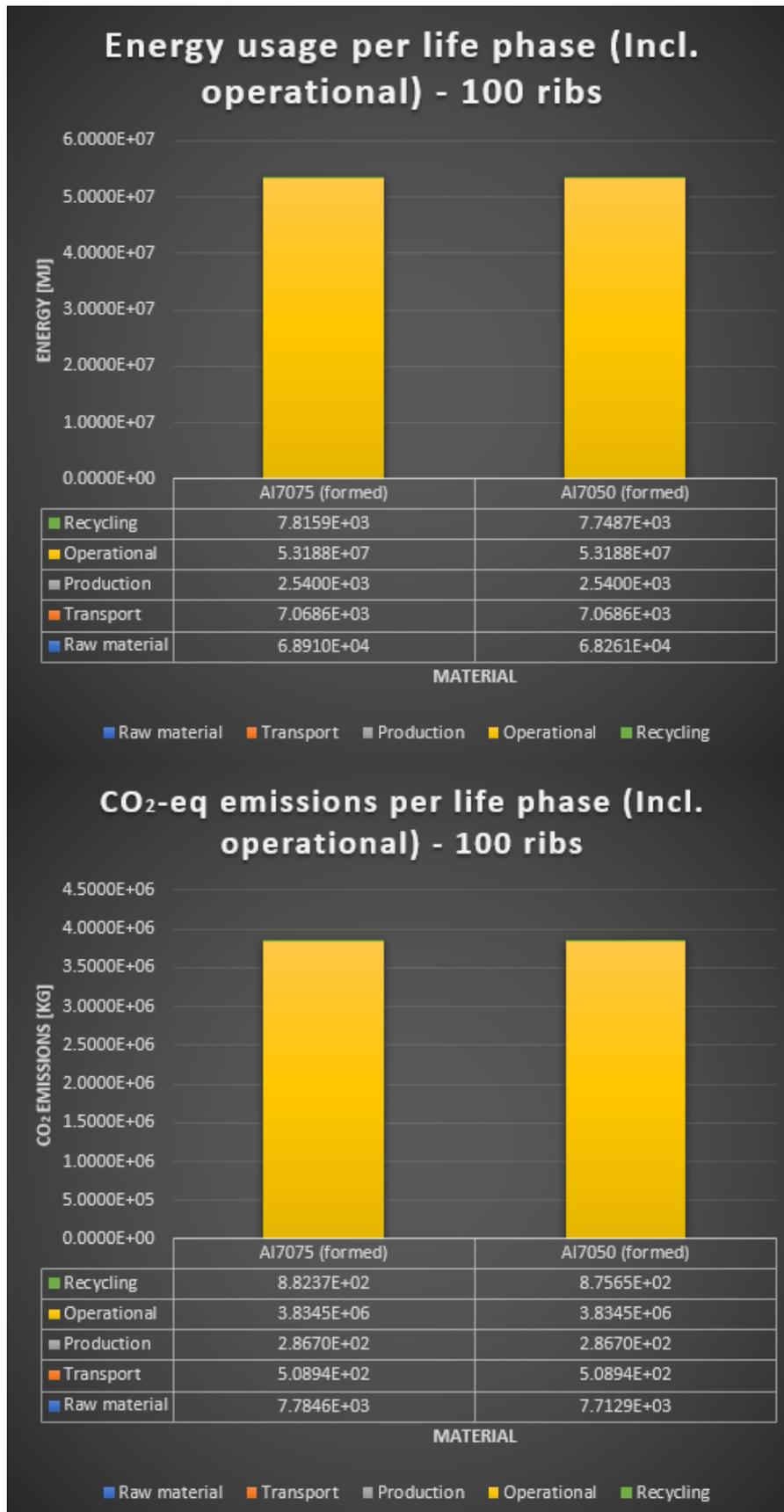
Figure 3.7: Sheet formed aluminium energy and CO<sub>2</sub> per life stage charts (including the operational phase)
