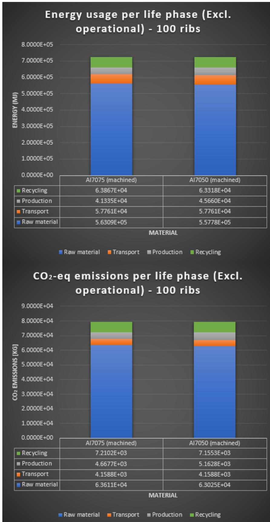
Figure 3.3: Machined aluminium energy and CO<sub>2</sub> per life stage charts (excluding the operational phase).
