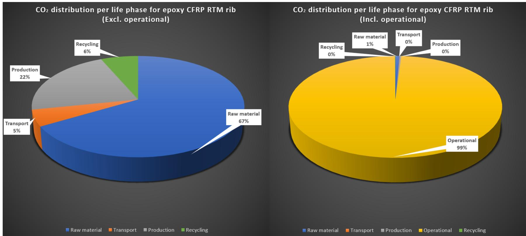
**Figure 4.8:** CO<sub>2</sub>-eq distribution per life phase for epoxy CFRP RTM rib
