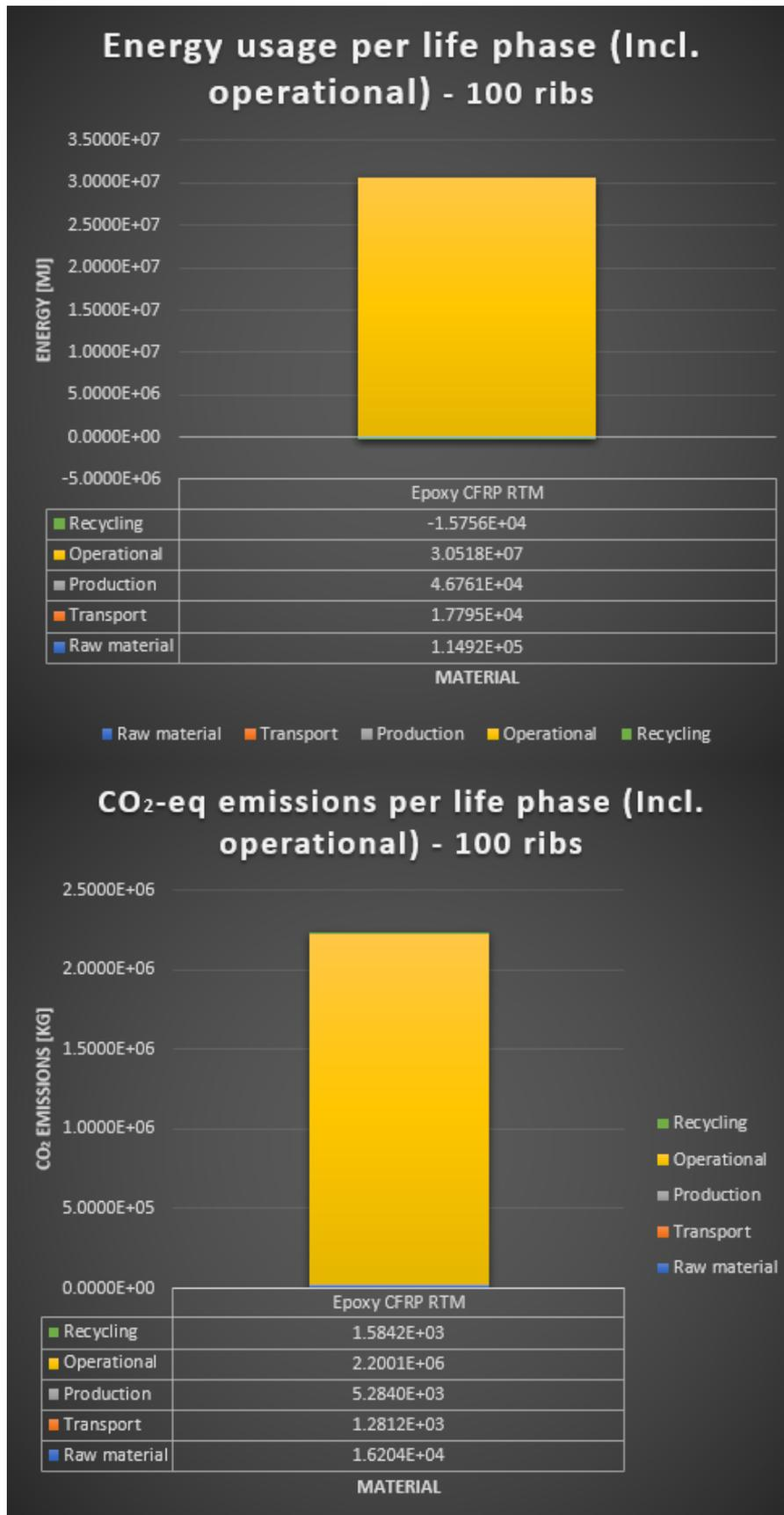
Figure 3.13: Epoxy CFRP RTM energy and CO<sub>2</sub> per life stage charts (including the operational phase)
