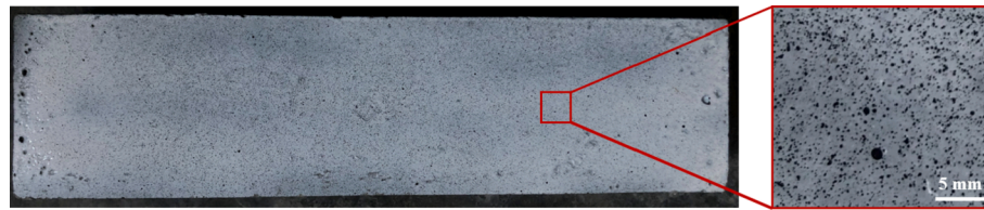
Fig. 1. Random speckle pattern obtained by black paint spray.
