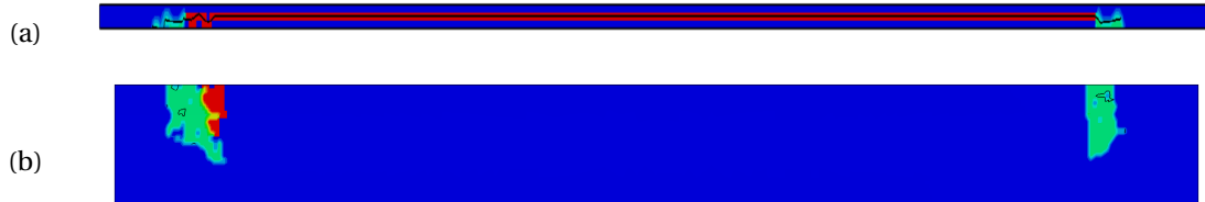
Figure 8.42: Predicted crack growth behaviour trough the interface section (deflection angle = 2.5°): (a) Cap-side view; (b)Bottom Surface
