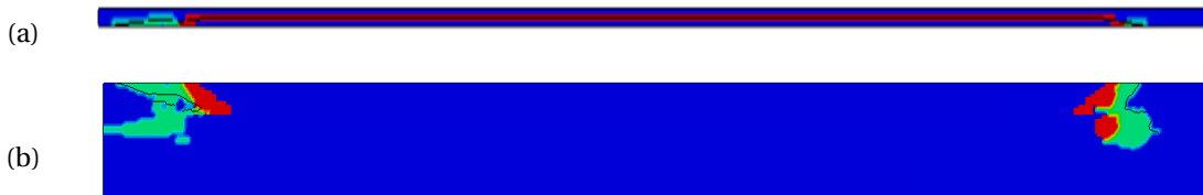
Figure 8.38: Predicted crack growth behaviour through the interface section (BIAS_FACTOR = 5): (a) Cap-side view; (b) Bottom Surface
