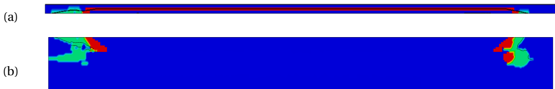
Figure 8.39: Predicted crack growth behaviour through the interface section (BIAS_FACTOR = 10): (a) Cap-side view; (b) Bottom Surface
