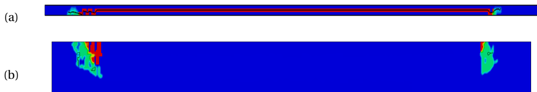
Figure 8.43: Predicted crack growth behaviour trough the interface section (deflection angle = 5°): (a) Cap-side view; (b)Bottom Surface
