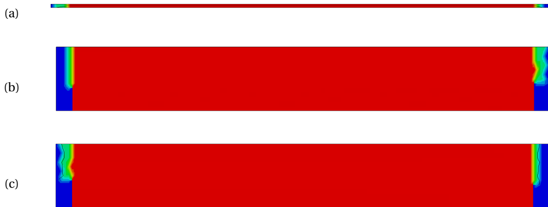
Figure 8.24: Predicted crack growth behaviour through the interface section: (a) Cap-side view; (b) Top Surface and (c) Bottom Surface
