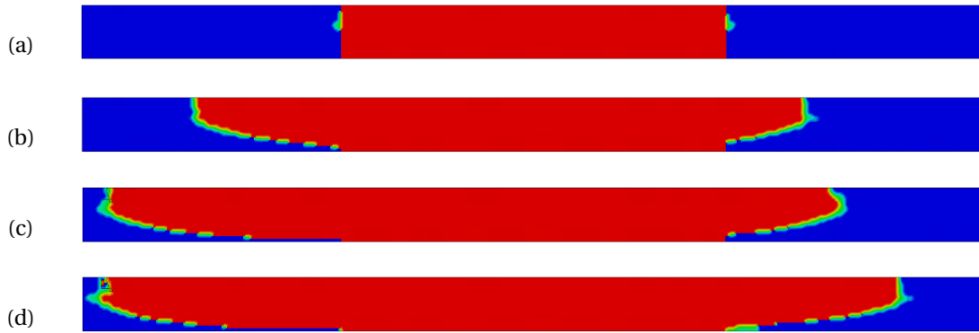
Figure 8.17: Evolution of delamination along the skin-stringer interface : (a) 116 kN; (b) 156 kN; (c) 192 kN and (d) Maximum Load
