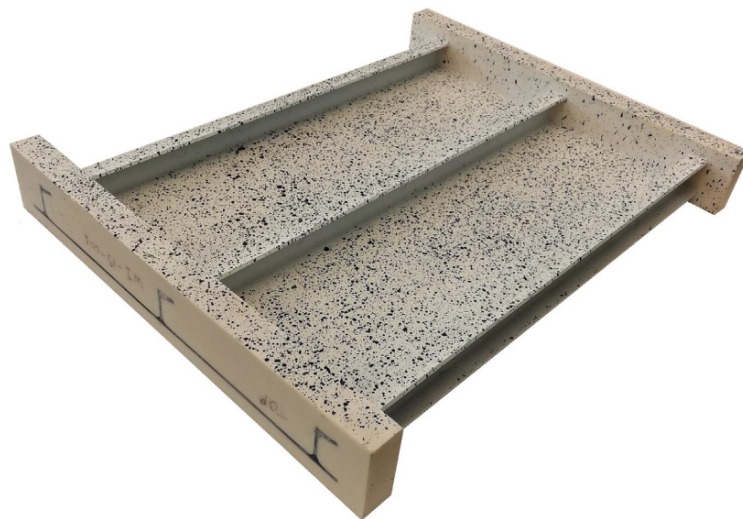
Figure 7.1: Thermoplastic Composite Stiffened Panel used by Dooren et al. for their study [50]
