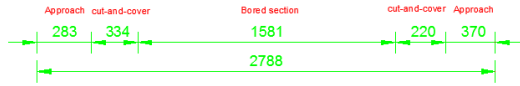
(a) Alignment of double tube bored tunnel without emergency lane with cut-and-cover section (Google map)
