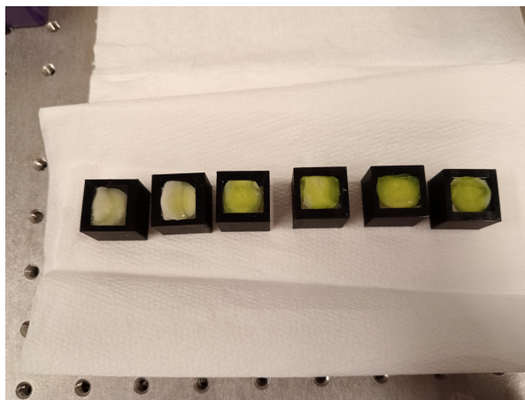
Figure 3.7: Six sensors used in the measurement where on each sensor a different pH buffer is deposited, ranging from the 6.2 pH buffer solution on the left to the 8.2 pH buffer solution on the right.
