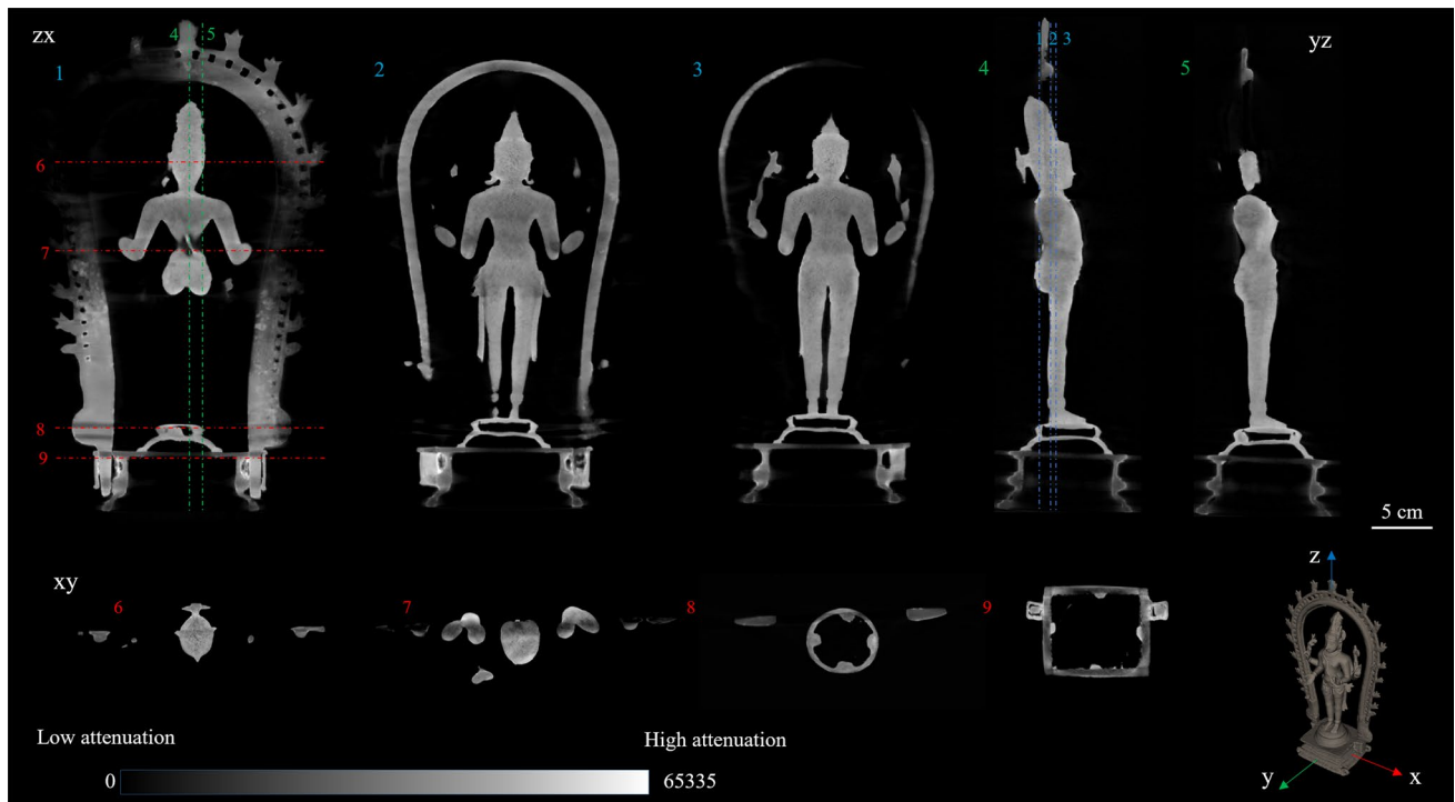
Fig. 2 Shiva (AK-MAK-1291). Neutron tomography projections. Normal slices ( zx ); sagittal slices ( yz ); axial slices ( xy )
