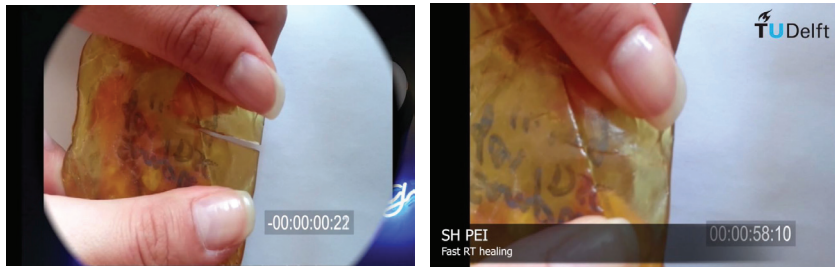
Fig. 20. Stills from a movie showing a self healing material, taken less than one minute apart.
