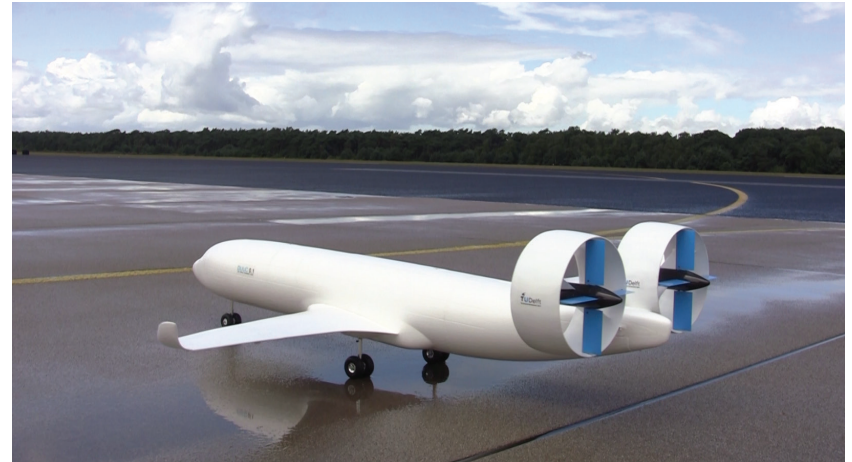
Fig. 22. Scaled flight testing of TU Delft aircraft concept
