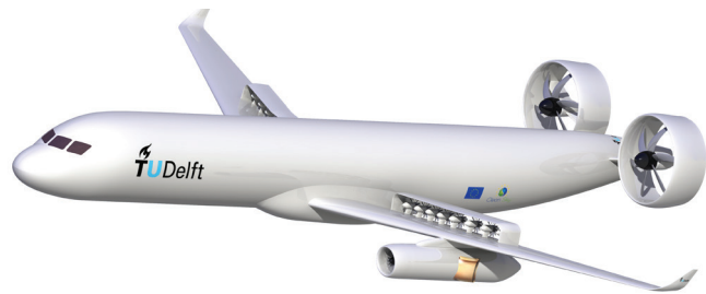
Fig. 15. Concept of a hybrid aircraft (turbines plus electric engines) developed at TU Delft.
