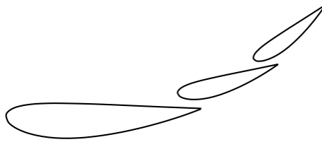
Figure 4: 3-element NACA 4418 wing configuration
