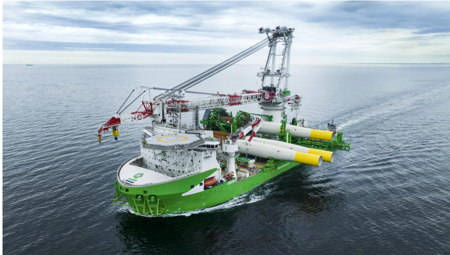
Figure 7.5: DEME Orion Vessel for XXL monopile installation
