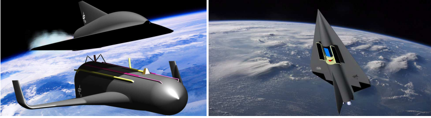
Figure 1.1: DLR SART – SpaceLiner 7. Left: SpaceLiner concept at stage separation with passenger stage in upper position. Right: Artist's impression of satellite payload release from SpaceLiner 7 Orbiter's open payload bay in low-Earth orbit (LEO). Credits: DLR, CC-BY 3.0. 1
