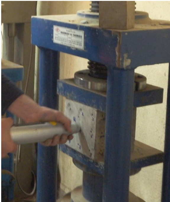
Figure 22: horizontal Schmidt hammer application
