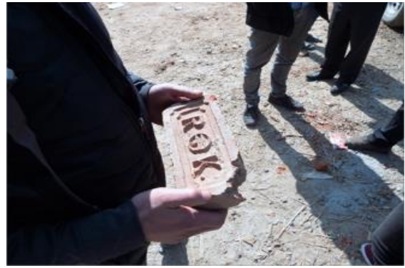
Figure 97: Damaged not-treated brick at the village of Pipaltar
