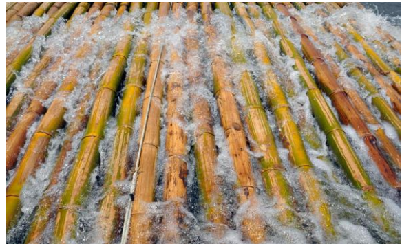
Figure 7: water leaching process, diminishing starch content of the material
