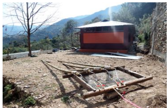
Figure 94: bamboo treatment with borax and boric acid and using gravity as pressure driving
