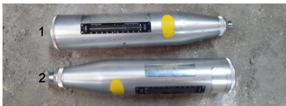
Figure 18: Schmidt hammers used for testing concrete blocks
