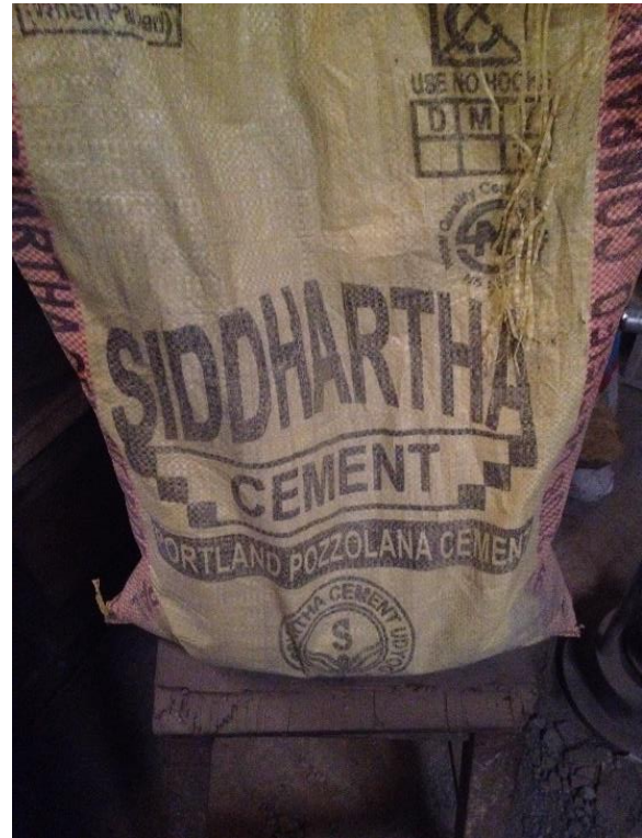
Figure 27: pozzolanic cement used to make the concrete in Ratankot
