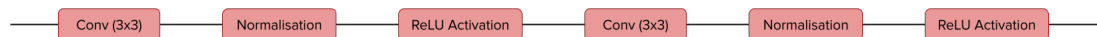
Figure 2.7: A VGG cell, that is also used in U-Net. It performs two convolution operations followed by normalisation and activation. It does not contain pooling or residual connections.
