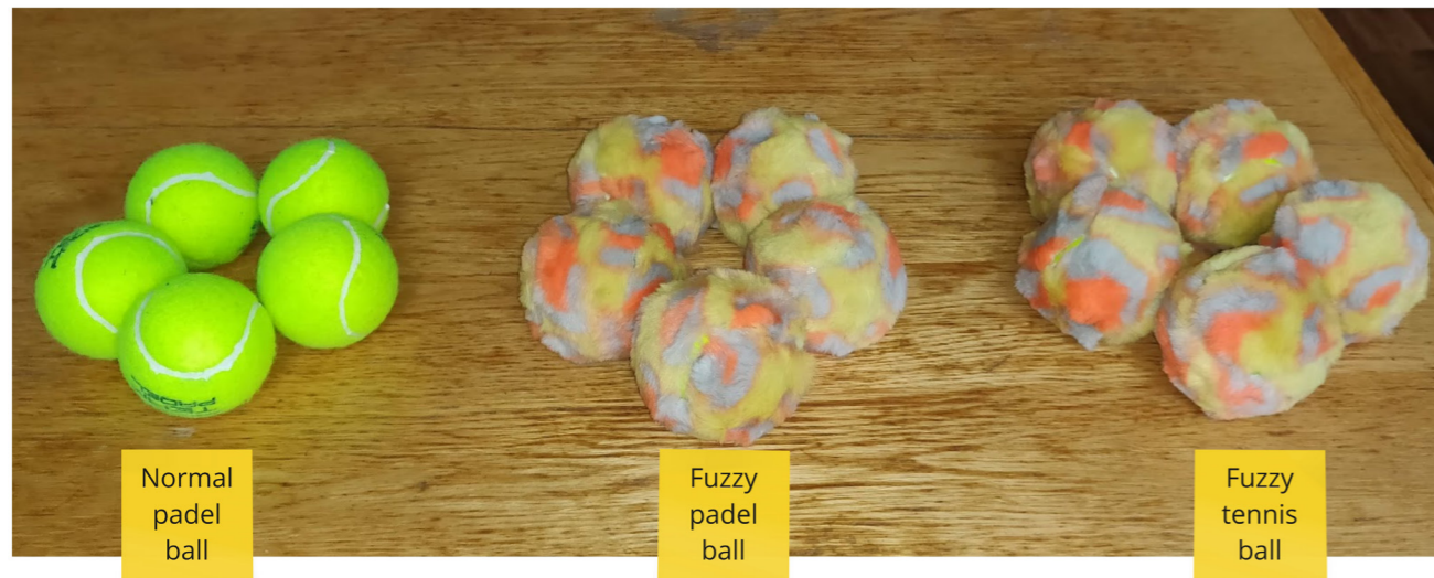
Figure 26: The balls used in the smash test; Pnormal (left), Pfuzz (middle), Tfuzz (right)
