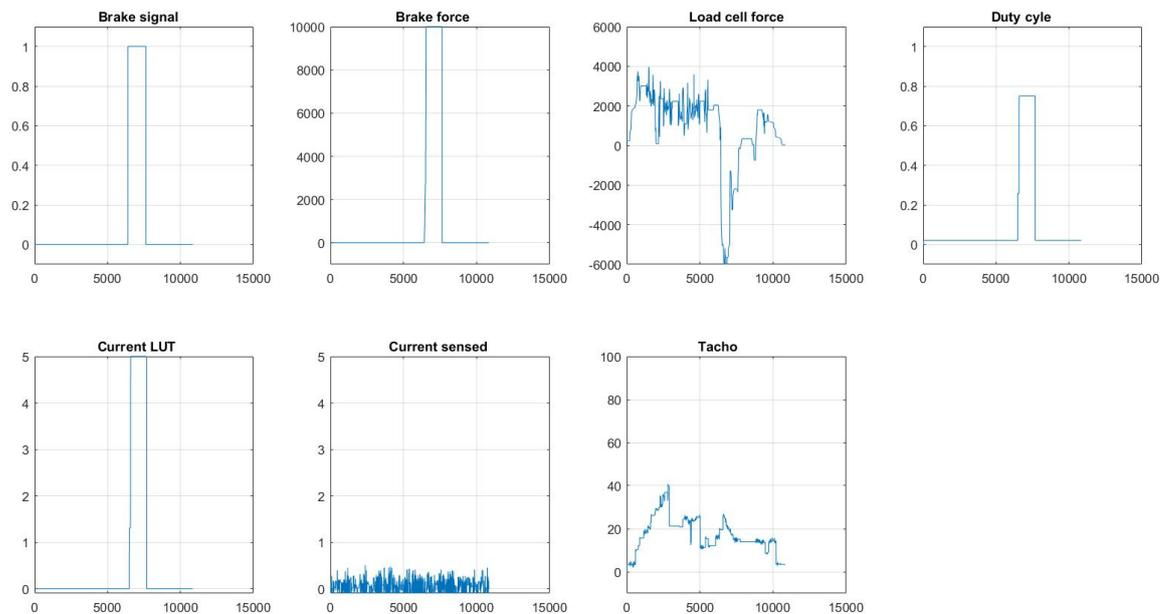
Figure 6.9: The braking session where the car makes an emergency stop.
