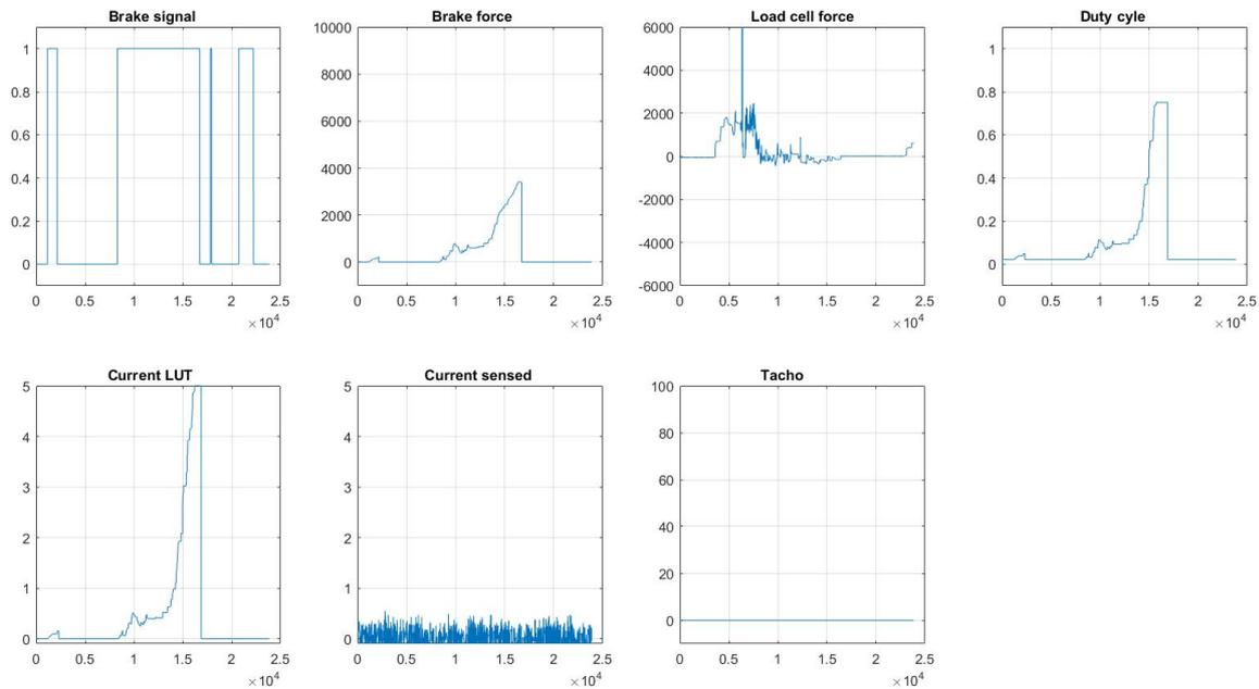
Figure 6.7: The braking session with the brakes activated. The brakes of the car brake lightly with increasing power.
