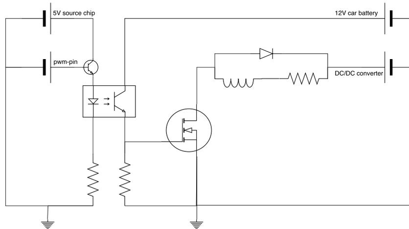
Figure 4.5: The total current control module circuit
