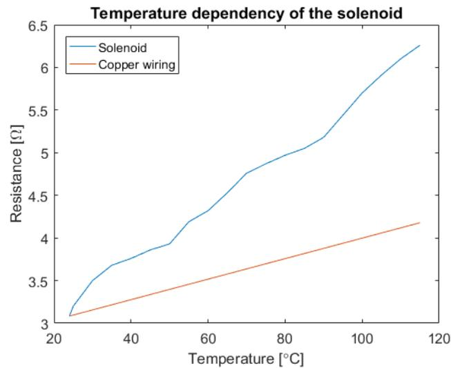
Figure 3.2: The resistance of the solenoid as a function of surface temperature.
