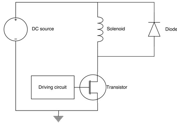
Figure 4.3: The topology of the current driving module
