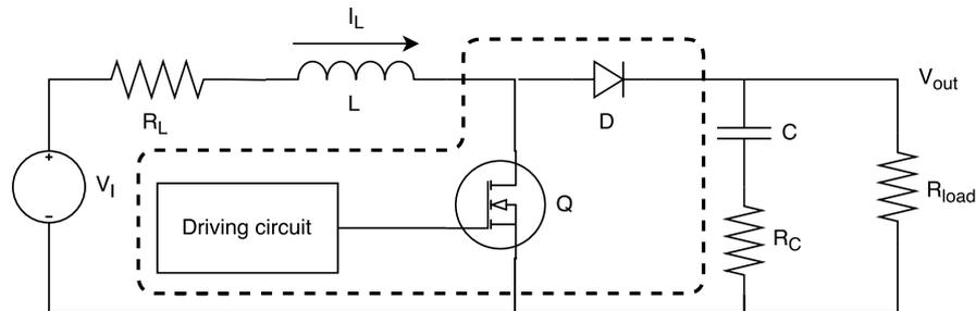
Figure 3.5: A standard boost converter topology.
