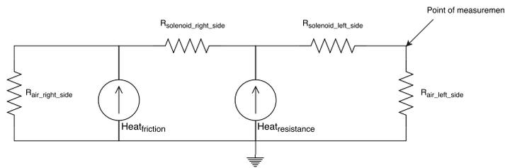
Figure 4.1: An electric analog of the heat convection
