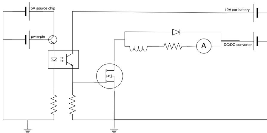
Figure 4.6: The total current control module circuit
