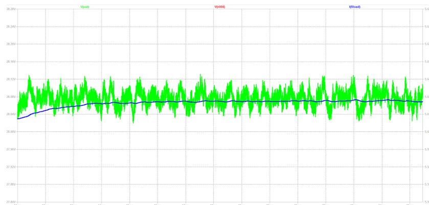
Figure 6.3: The current and voltage ripple at the output of the converter.
