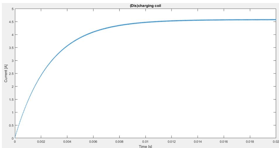
Figure 6.4: Charging the solenoid with a switching frequency of 20 kHz
