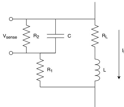
Figure 3.7: The DCR sensing circuit.
