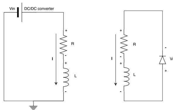
Figure 4.4: The circuits belonging to the ON(left) and OFF(right) state of the MOSFET
