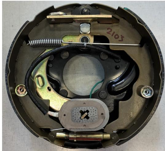
Figure 5.1: The used drum brakes in the E-Brake system.
