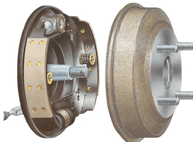
Figure 5.2: The drum and the inner side of a regular hydraulic drum brake [22].
