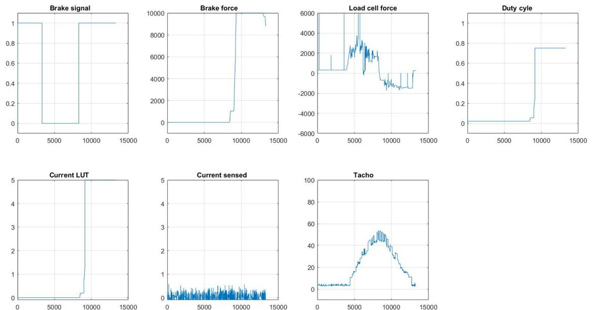
Figure 6.6: A braking session where the brakes are decoupled from the circuit.
