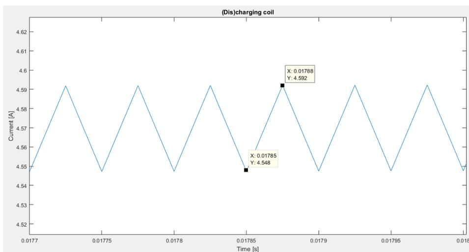
Figure 6.5: The current ripple at displayed at the switching frequency of 20 kHz
