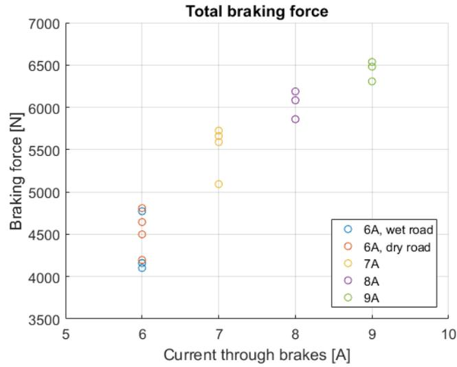
Figure 3.1: The braking force of two drum brakes installed on a single axle trailer.
