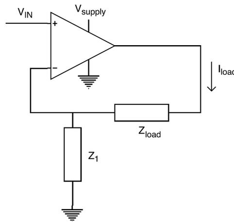
Figure 3.3: A basic voltage to current amplifier topology
