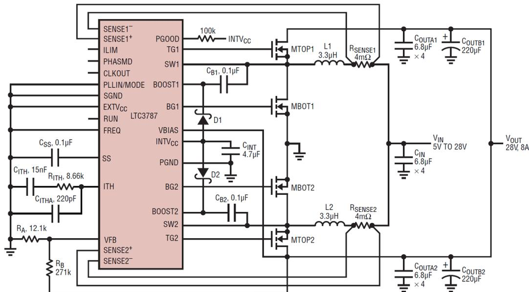
Figure 3.6: The 2-phase synchronous boost converter topology [19].
