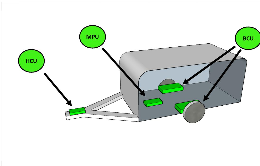
Figure 1.1: An overview of the subsystems in the trailer.
