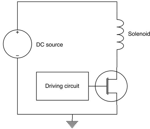
Figure 3.4: The transistor topology.
