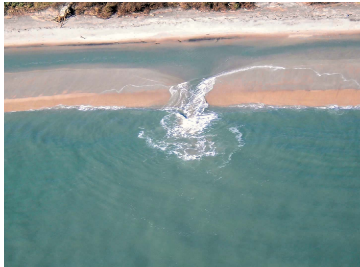
Figure 2-2: Rip current formed between sandbars, https://www.britannica.com/science/rip-current
