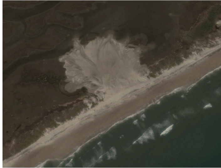
Figure 2-3: Overwash on Onslow Beach, North Carolina, USA, March 2013, screenshot from Google Earth.
