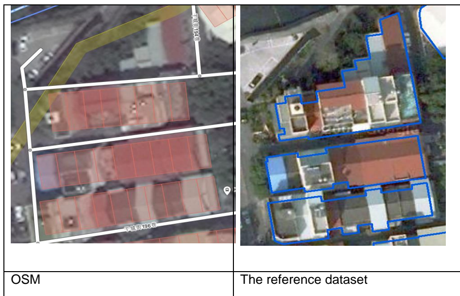
Figure 9: The OSM building footprints have higher resolution than the reference dataset in Taichung (Base Map ©2016 Bing, ©2016 Google)
