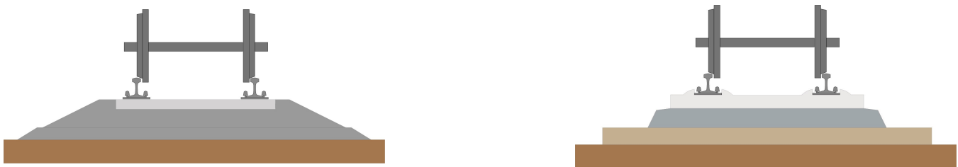
Figure 1: Ballasted and slab track respectively from left to right (TU Delft, n.d.)
