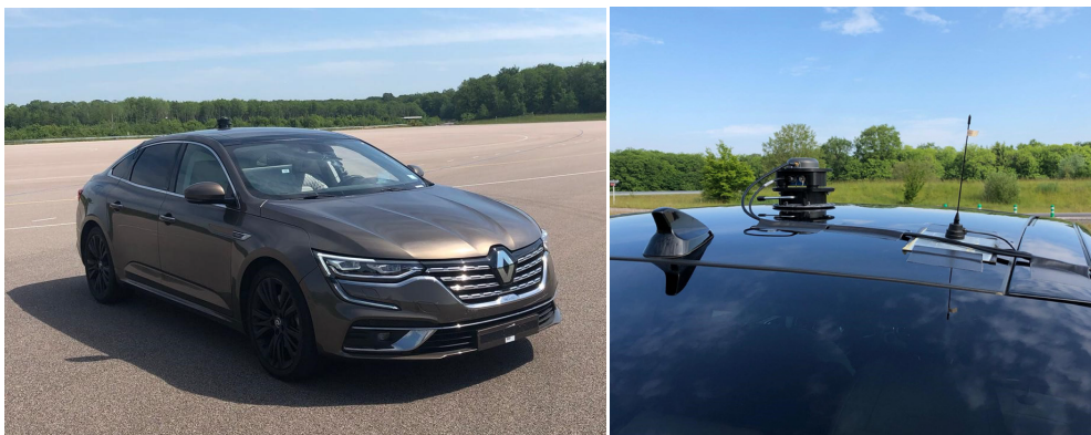
Figure 7.1. The experimental vehicle, a Talisman phase 2 (left), with the VBOX GPS antenna (right)
