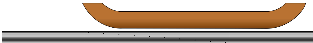
Figure 4.25: First position of the coil used to weld the STI specimen
