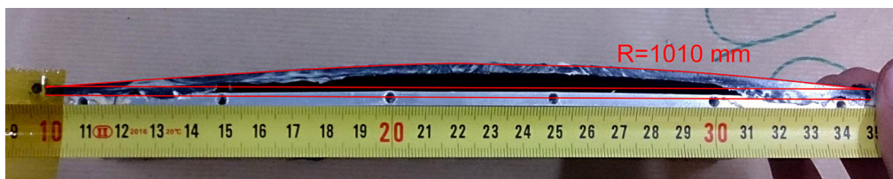
Figure 4.31: Compressed CTP specimen after consolidation before unloading
