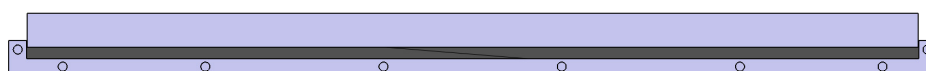
Figure 4.30: Schematic side view of the press join tool with circles indicating the location of the screws used to attach the sides
