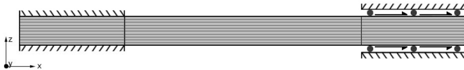
Figure 5.11: Boundary conditions used in the FEM model
