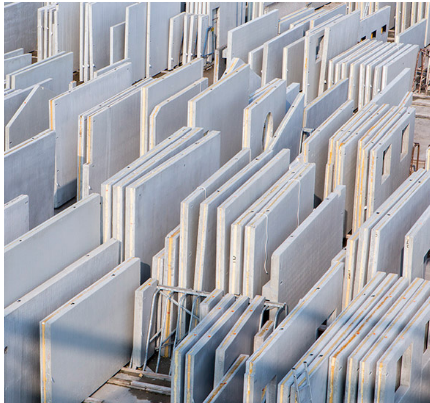
demountable prefab concrete elements for cores
