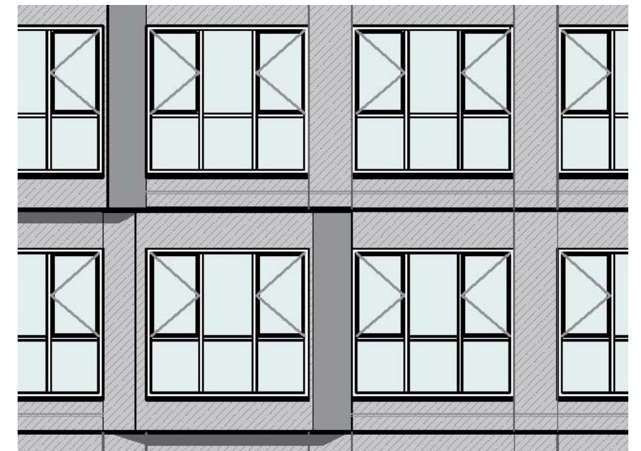
modular facade elements (as it was in the existing building)
