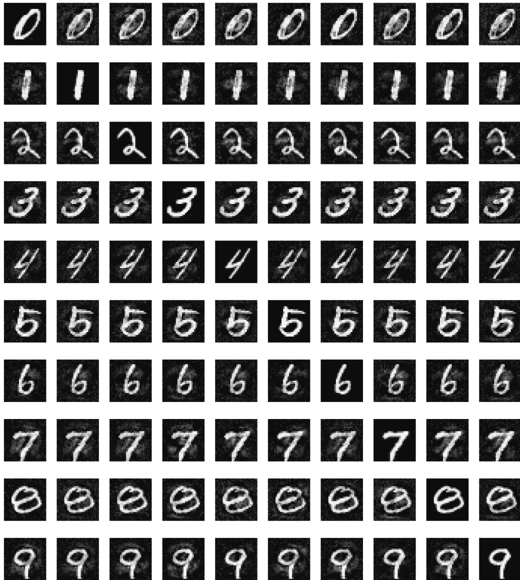
Figure 7: Table with counterfactuals generated with a deep ensemble and the ECCo generator. The factuals are positioned along the main diagonal of the grid, the number of the row is the original label of the factual, while the number of the column shows the target of the label
