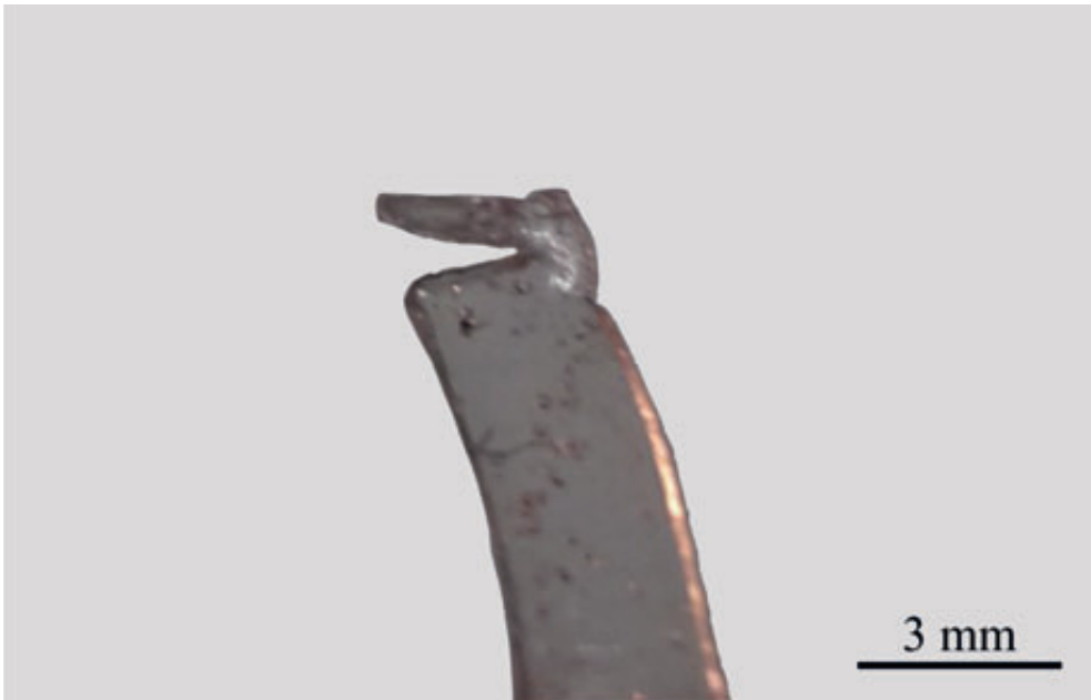
Figure 13.14 — Incomplete resection of the gelatin phantom with the beveled blade design.
