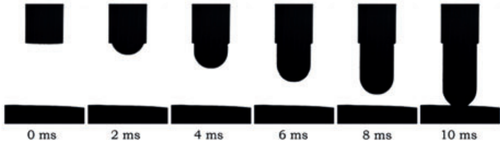
Figure 7.11— Example of an HSV Image Sequence of an Indenter Strike with an Object Distance of 3 mm and a Spring Compression Distance of 3.5 mm. An average indenter velocity of 3.0 m/s can be derived.
