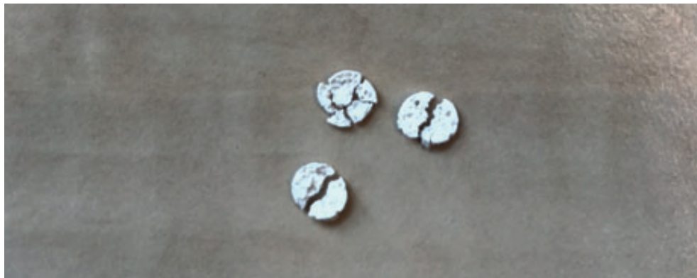
Figure 8.14— Typical punctures of the proximal model.
