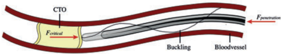
Figure 10.1— Buckling of the Guidewire During the Endovascular Treatment of CTOs. The guidewire is pushed from outside the body against the CTO (yellow) using a penetration force ( F_{penetration} ). The CTO exerts an opposite compressive force onto the guidewire until puncture is achieved at approximately 1.5 N according to Thind et al. [6]. If the compressive force exerted by the CTO exceeds the critical buckling load ( F_{critical} ) of in between 0.008–0.26 N depending on the guidewire, buckling of the guidewire tip, indicated by the dark grey line, will occur.
