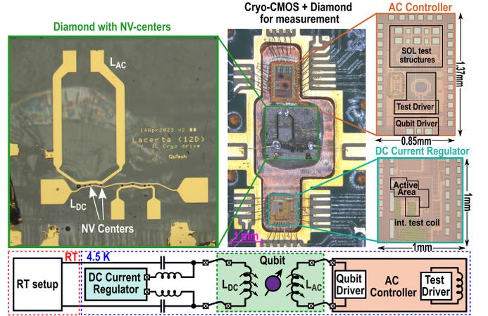
Fig. 11. Integrated cryo-CMOS and NV-center SIL sample. Two gold striplines,  $L_{AC}$  and  $L_{DC}$ , are patterned on the diamond.  $L_{DC}$  is bonded to a bias-T, which combines the DC CR and the RT setup.  $L_{AC}$  is directly bonded to the AC controller. The AC controller chip also hosts a test driver with an on-chip coil and short-open-load (SOL) test structures to characterize the driver and on-chip coil.
