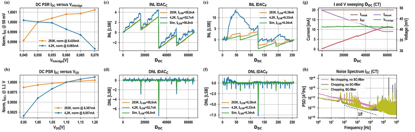
Fig. 14. Electrical characterization of the DC CR at RT (293 K) and CT (4.2 K). (a) and (b) show the DC PSR versus  $V_{H\text{-bridge}}$  and  $V_{DD}$ . (c) and (d), and (e) and (f) show the INL and DNL of the  $IDAC_C$  and  $IDAC_F$ , respectively. (g) shows the operation of the DC CR with shunt path enabled. (h) shows the noise PSD at CT. Simulations are done at 300 K
