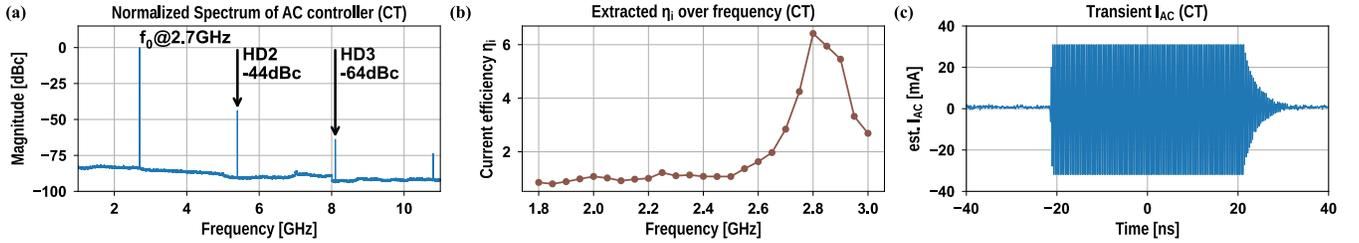
Fig. 12. Electrical characterization of the AC controller: (a) normalized spectrum measured with the magnetic probe; (b) extracted current efficiency  $\eta_i = I_{AC}/I_{DC,driver}$  over frequency; and (c) transient waveform of  $I_{AC}$  extracted with the magnetic probe.
