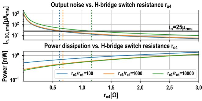
Fig. 9. Sweeping noise and power as a function of  $r_{o4}$  and  $r_{o3}/r_{o4}$ , the black line indicates the allowed noise for 99.9% fidelity and the colored dashed lines indicate the  $r_{o4}$  for which the noise requirement is met.
