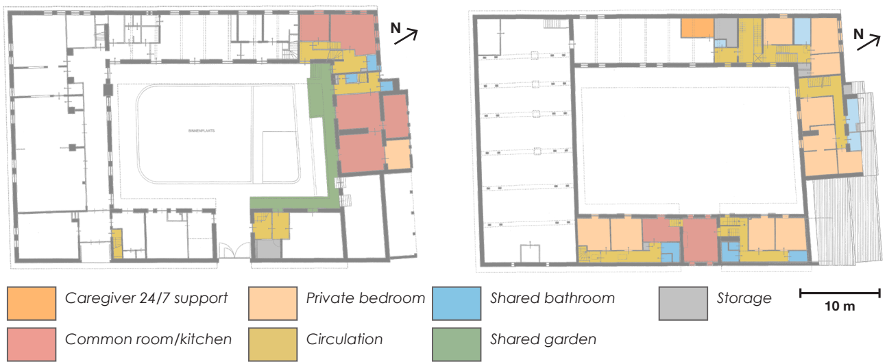
Figure 19: Floorplans of the main farm building on location C with focus on the group housing (ground floor on the left, first floor on the right)
