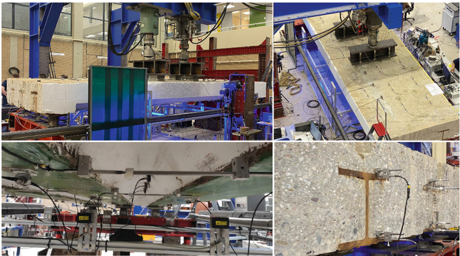
Fig. 5. Test and instrumentation. Top Left: side overview; Top Right: top view and optic fibers. Bottom Left: Bottom view transverse LVDTs; Bottom Right: Side view end LVDTs.
