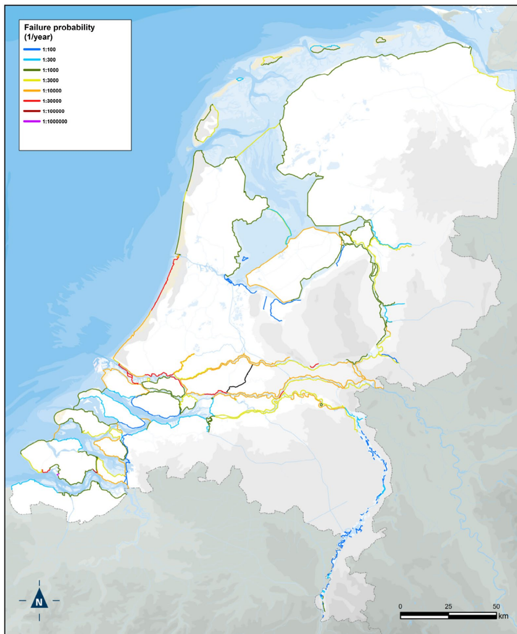
Figure 4. New safety standards for flood defences in the Netherlands, in the form of maximal acceptable failure probabilities (Ministerie van Infrastructuur en Milieu, 2016a). Source: Public information from the Dutch government (Rijkswaterstaat).
