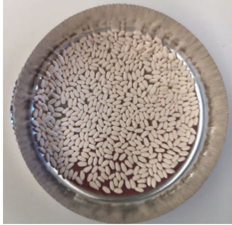
Fig. 1. Printed zeolite granules (after sintering at 950 °C)
