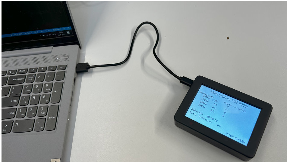
Figure B.2: The UI screen functionality was developed using a test setup created by our colleague Rik Imbens. The laptop is connected via USB to the test setup. The circuit used in the Control Unit is the same as that from the test setup
