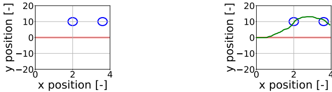
Fig. 12. Setup used in the 2D example, the blue circles and red line represent the viapoints and predicted trajectory respectively. Left: Initial model trained at \vec{s} = [0, 0] , which fails to reach the viapoints. Right: Refinement created using teleoperation, depicted as a green line
