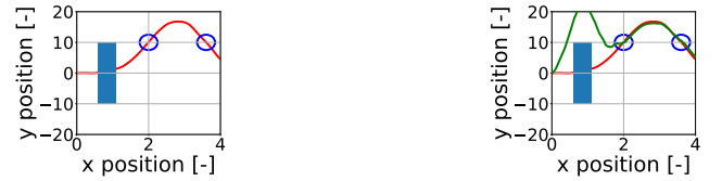
Fig. 13. Prediction and refinement with an obstacle, the red and green trajectory are the prediction and refinement respectively.
