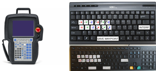
Fig. 17. Left: Teach pendant, Right: Implemented representation of the teach pendant using a keyboard
