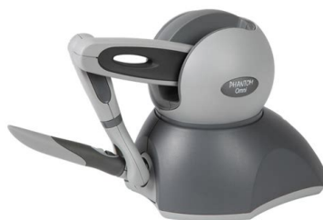
Figure C.1: Phantom Omni device used to generate the initial demonstrations
