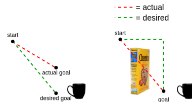
Fig. 1. Left: Goal deviation due to sensor inaccuracies, Right: Unforeseen obstacle
