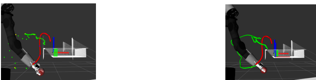
Fig. 29. Result of using different interpolation points, on the left and right image 75 and 500 interpolation points are chosen respectively
