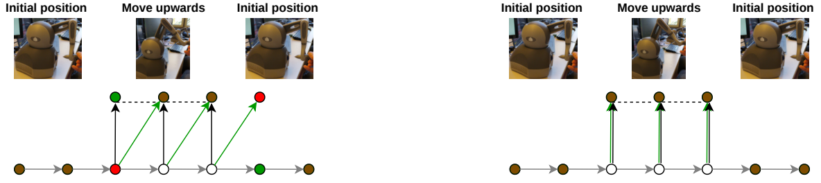
Figure B.18: Left: Adaptation of the next time step, Right: Adaptation of the current time step. The green and red dots represent the master and slave position respectively, and when they are on the same position, the dot is indicated as a brown color. The white dot represents the reference trajectory, where the executed trajectory converges to if the operator does not apply any input.
