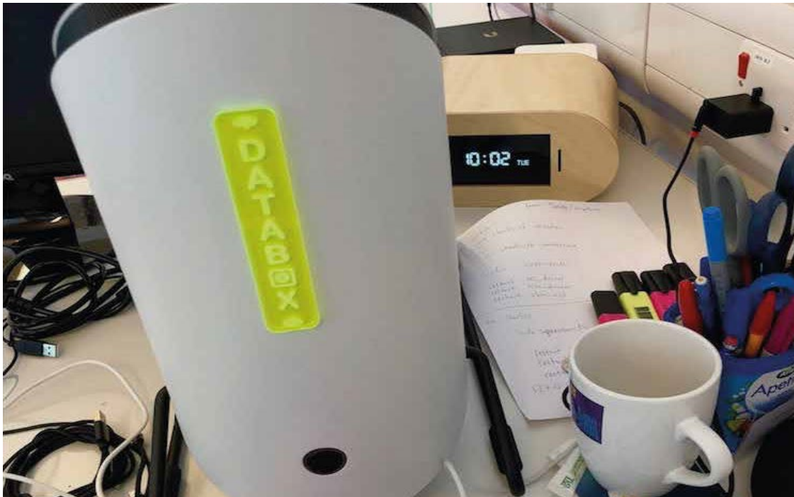
Figure 2 The Databox home router is an Edge IoT data processing device ( www.databoxproject.uk ).
