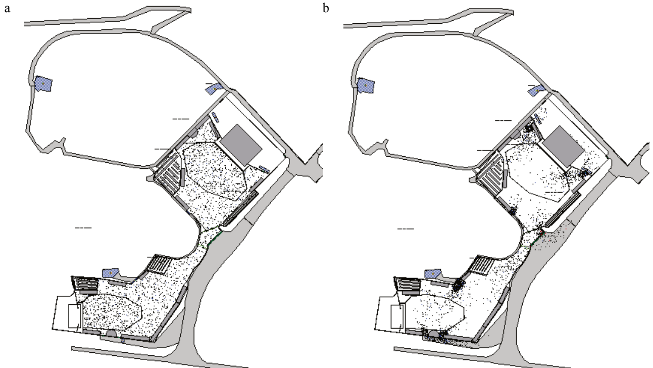
Fig. 6. Visualization of the evacuation of an event terrain. (a) At the start of the evacuation; (b) During the evacuation.
