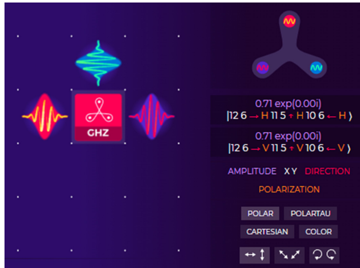
Fig. 10 A three-particle Greenberger–Horne–Zeilinger entangled state, visualized simultaneously as (A) waves on the board, (B) entanglement between particles, and (C) the quantum state, in bra-ket form.
