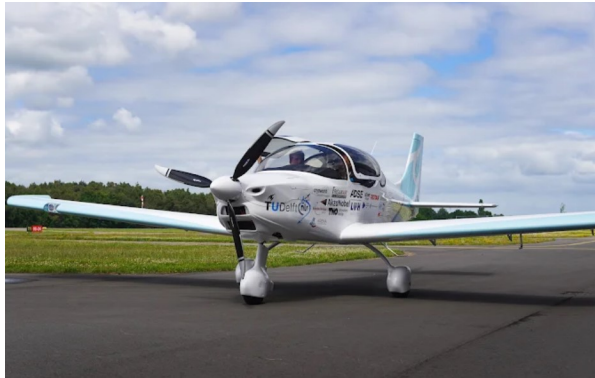
(a) AeroDelft's retrofitted Sling 4 hydrogen-powered electric aircraft [7]
