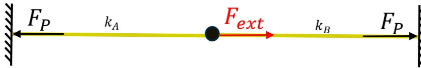
Figure 6.10: Simplified rope setup illustrating the effect of rope preload
