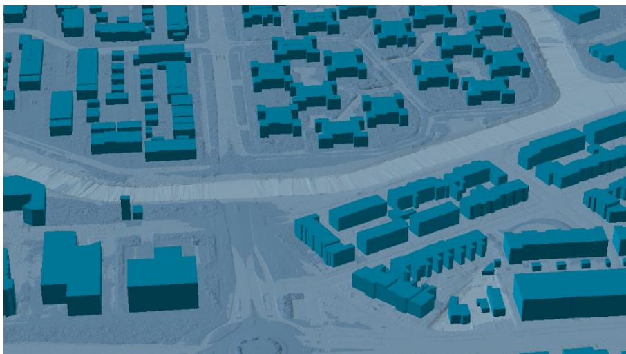
Figure 4. 'Model 2' digital terrain model produced with ground level points of AHN3
