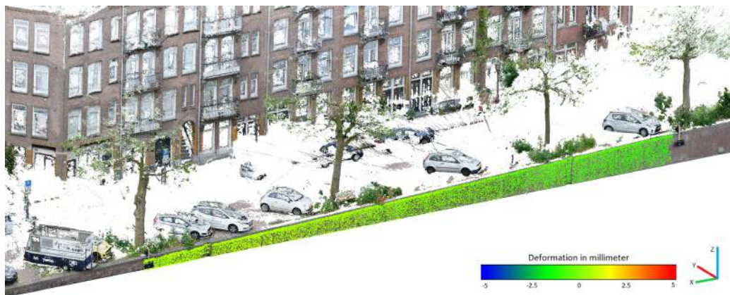
Figure 4.10: Point cloud with deformation points. The deformation points are coloured to the deformation in Z direction, which is the direction vertical along the quay wall. The position of the reference plates with control are indicated with an arrow.
