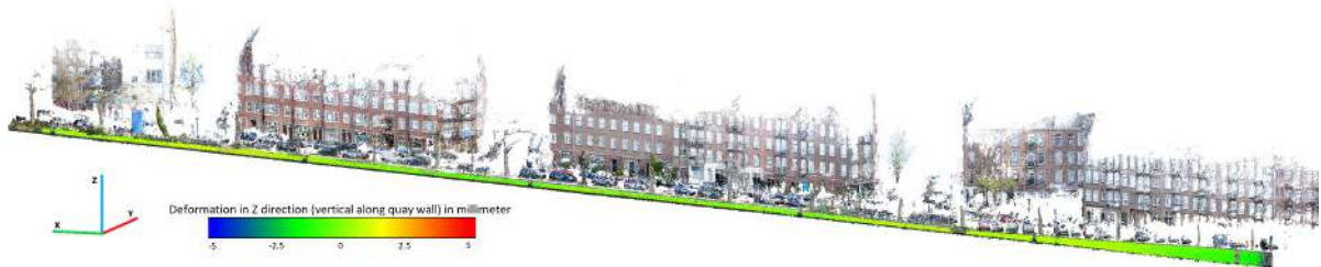
(c) Estimated Z-deformation between epoch 3 and 4
