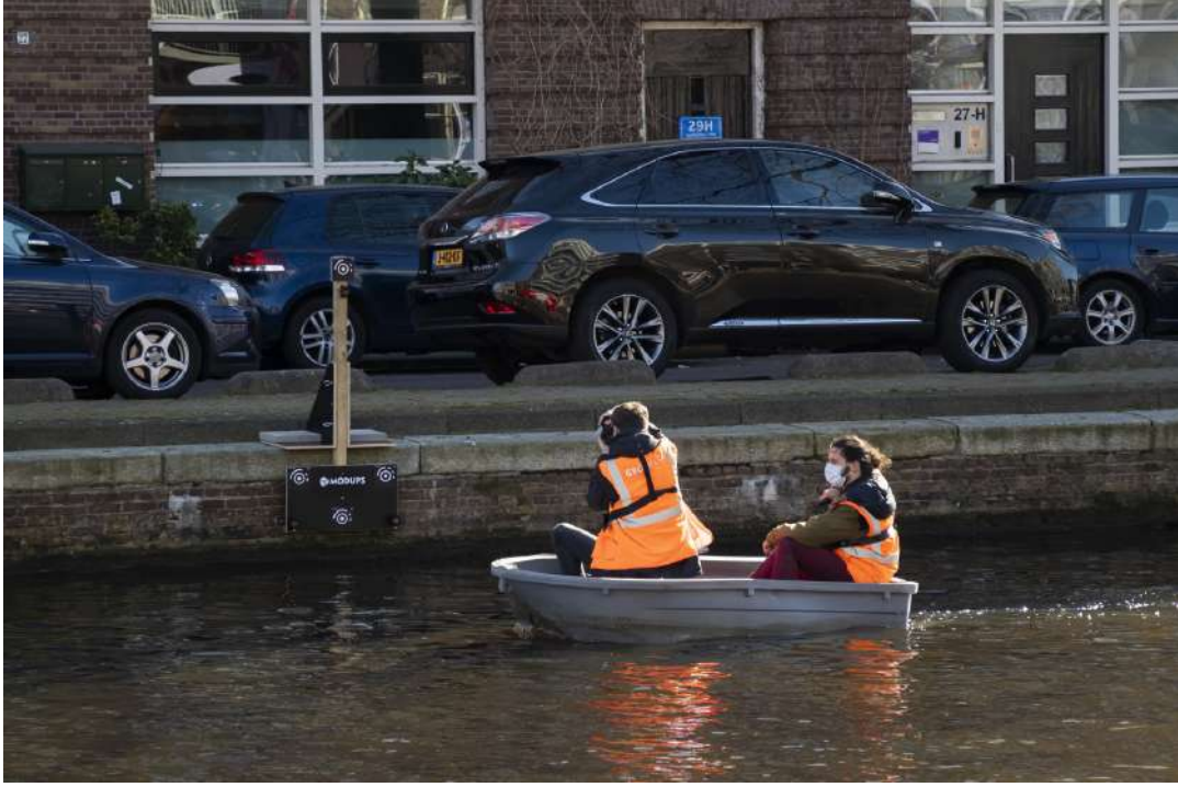
Figure 3.4: Picture of the process of imaging the the quay wall. The boat is sailing parallel to the quay wall at approximately 5 meter distance.
