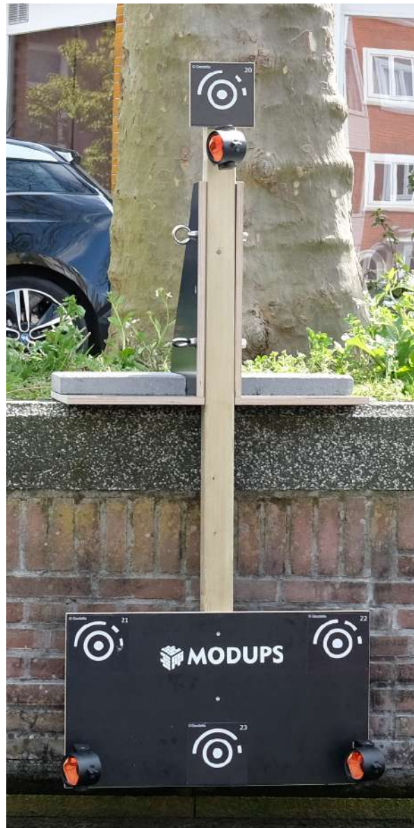
Figure 3.2: A reference plate for the photogrammetric measurements. The reference plate has four round barcode markers, which have a numbering and can be pinpointed using computer vision. Also there are three orange prisms present, which are very accurately and reliably measurable by tacheometer.
