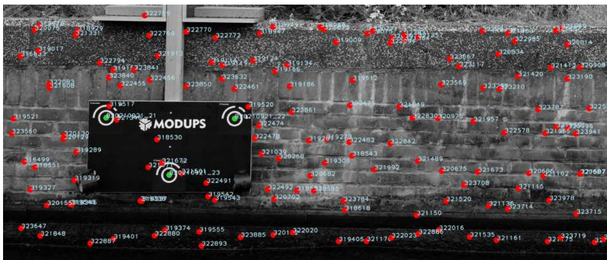
Figure 4.13: Part of an image used in the deformation analysis with some observations plotted in the image. Observation positions are presented as coloured dots with a name in the image. The name is used so an observation of the same point is identifiable in multiple images. Sift observations are the red dots and barcode observations are the green dots. The image has been turned to grayscale to make the coloured dots and labels more visible. The image has more more observations than shown, however plotting all observations will impede the clarity
