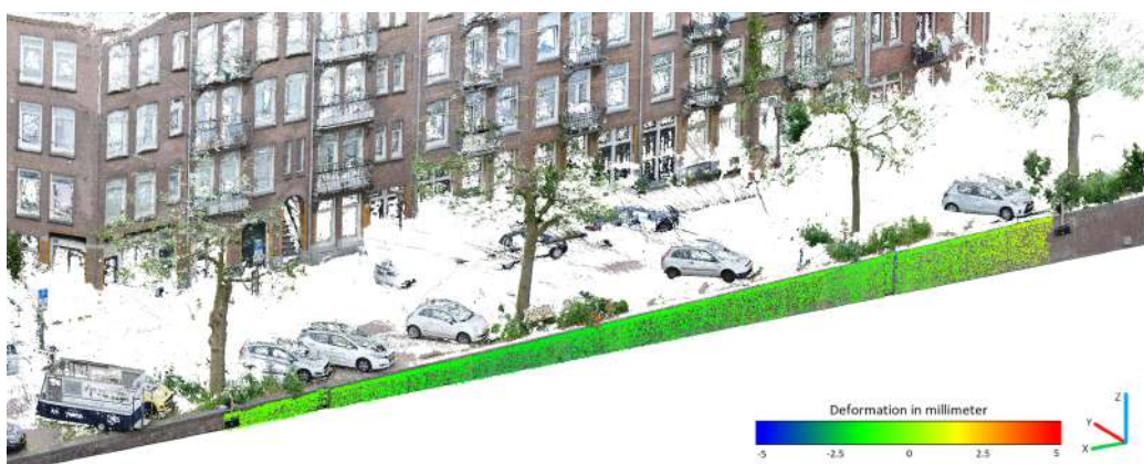
Figure 4.8: Point cloud with deformation points. The deformation points are coloured to the deformation in X direction, which is the direction horizontal along the quay wall. The position of the reference plates with control are indicated with an arrow.
