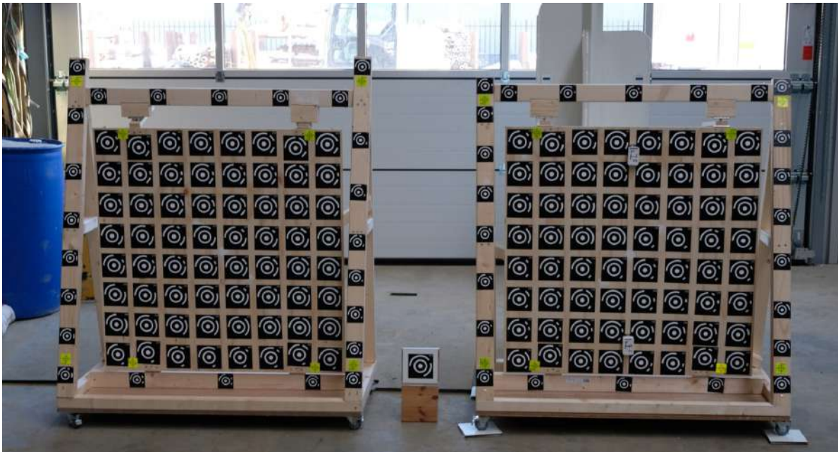
Figure 4.1: Mock quay wall test setup. The two wooden boards represent a quay wall. The boards are moved and tilted by which a deformation is simulated.
