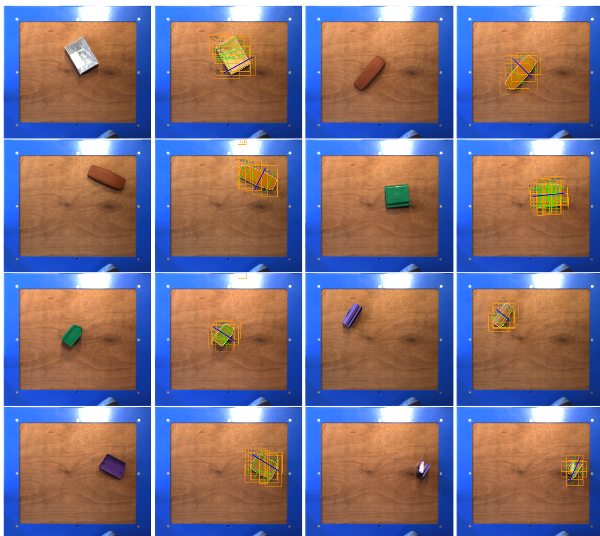
Figure C.1. Grasp predictions for images from experiment 1. The first and second column are the RGB images. The second and fourth column contain the predictions. The predicted pixels of the objects are covered yellow, the predicted grasps are given in green and the grasp that is executed is shown in blue.
