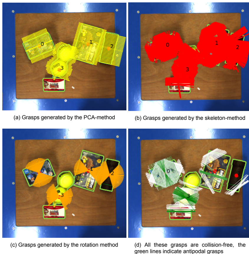
Figure 2.11. The grasps generated by the annotation tool on actual data are based on (a) the PCA method, (b) the skeleton method, and (c) the rotation method. After the grasp generation, the grasps are checked for collision with surrounding objects. It is also checked if the grasps are antipodal. Figure 2.11d shows all collision-free grasps in white and green. Grasps that are antipodal are indicated in green and are saved to train the network.
