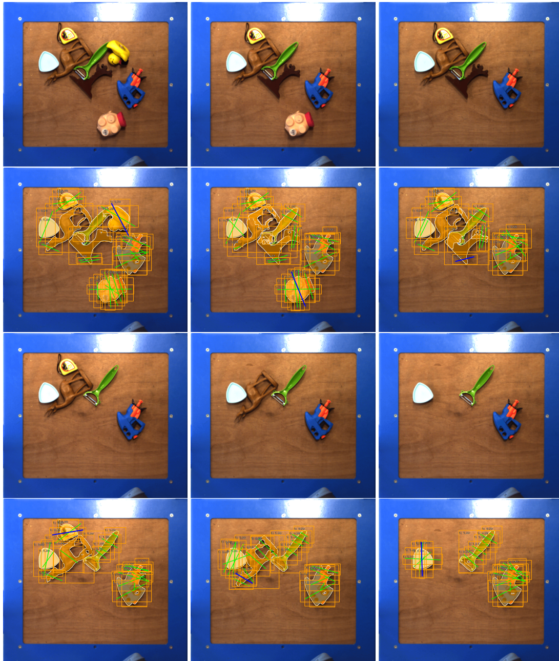
Figure C.2. A sequence of grasps of experiment 2. The first and third row contain the RGB image at the grasp area. The second and fourth row gives the predictions by the grasp network. The predicted pixels of the objects are covered yellow, the predicted grasps are given in green and the grasp that is executed is shown in blue. Sequence: Rubber duck, Piggy Bank, Wooden Tree, Measuring Tape, Wooden deer and a Triangle box.
