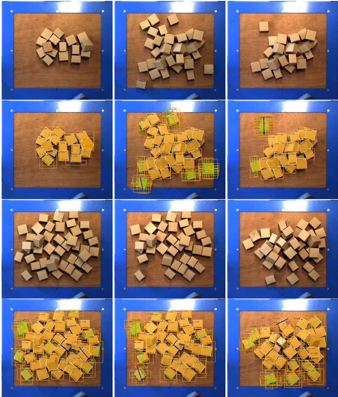
Figure C.3. Network predictions from experiment 3. The first and third row contain the RGB-image at the grasp area. The second and fourth row gives the predictions by the grasp network. The predicted pixels of the objects are covered yellow, the predicted grasps are given in green and the grasp that is executed is shown in blue.
