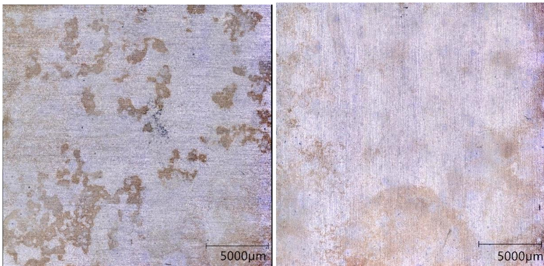
Figure 5.35 Surface images of Ref_pH4 (left) and NaGal_pH4 (right).
