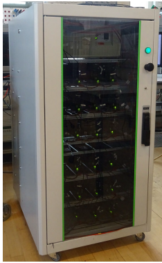
FIGURE 7. Laboratory prototype of MMC DS-STATCOM.
