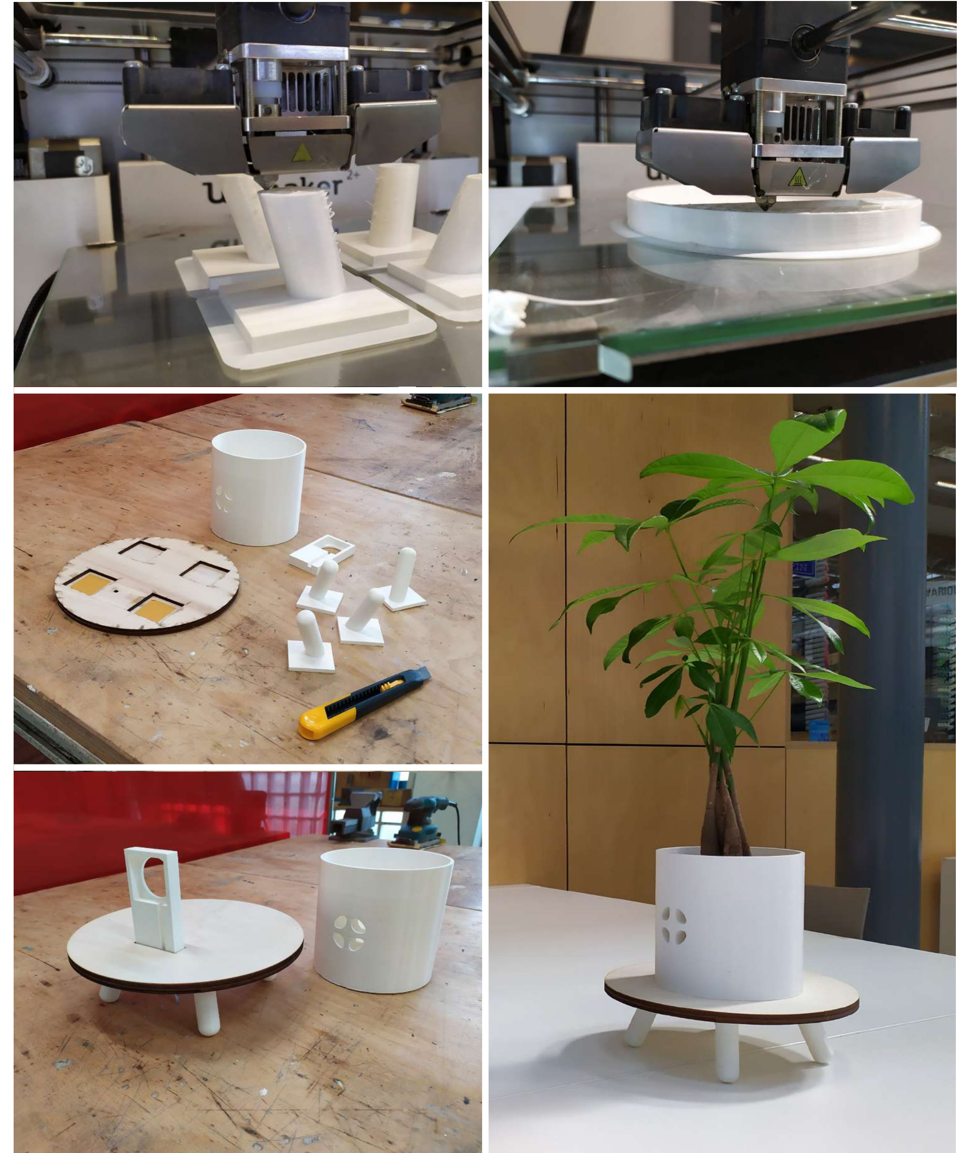
Figure 50 . Prototyping of a first model to get an idea about the product's size
