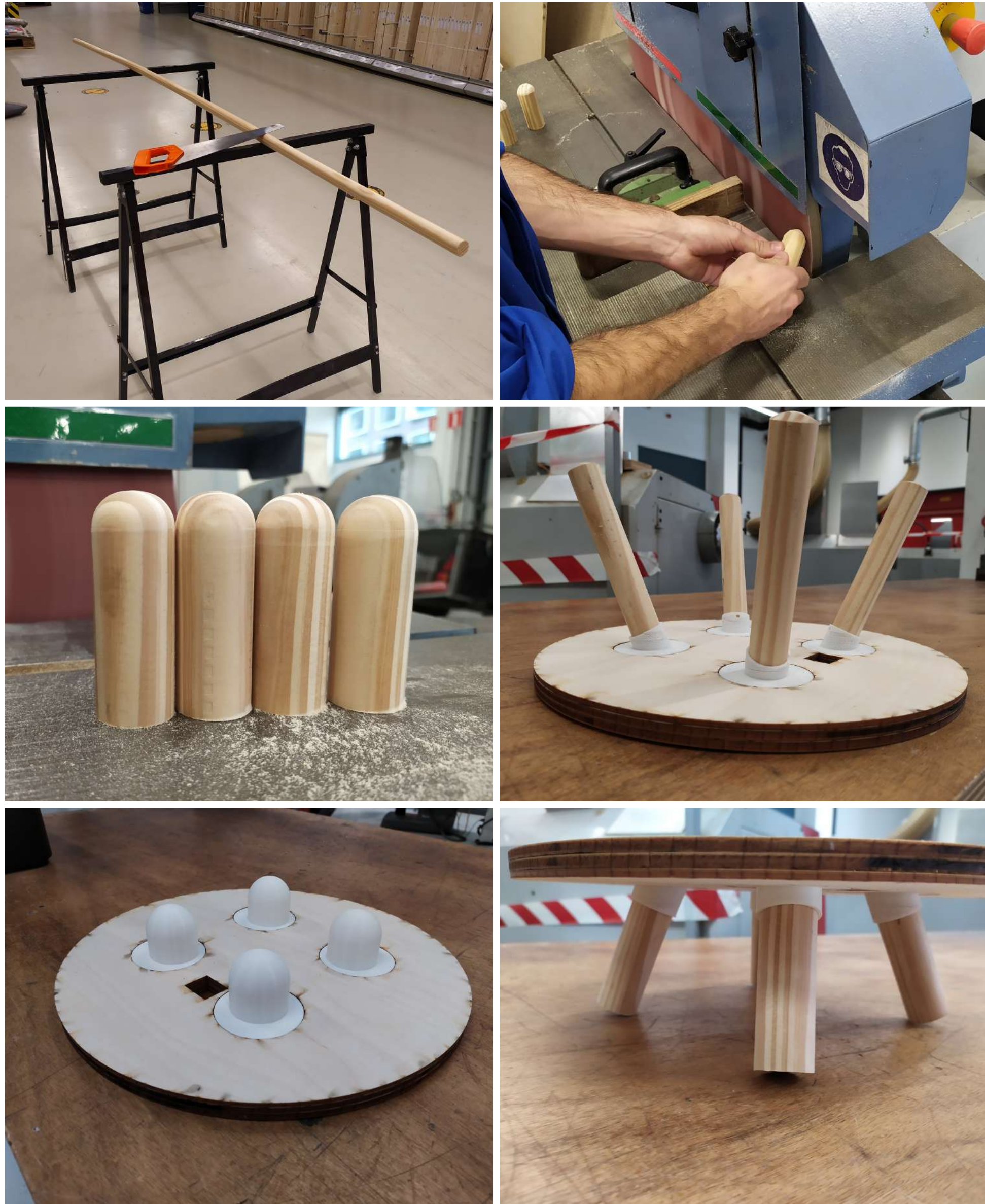
Figure 53. Prototyping with wood and 3D printing to explore different legs options
