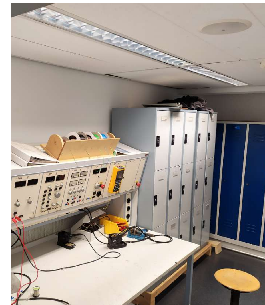
Figure 13. Artificially illuminated workplace: 638 lx
