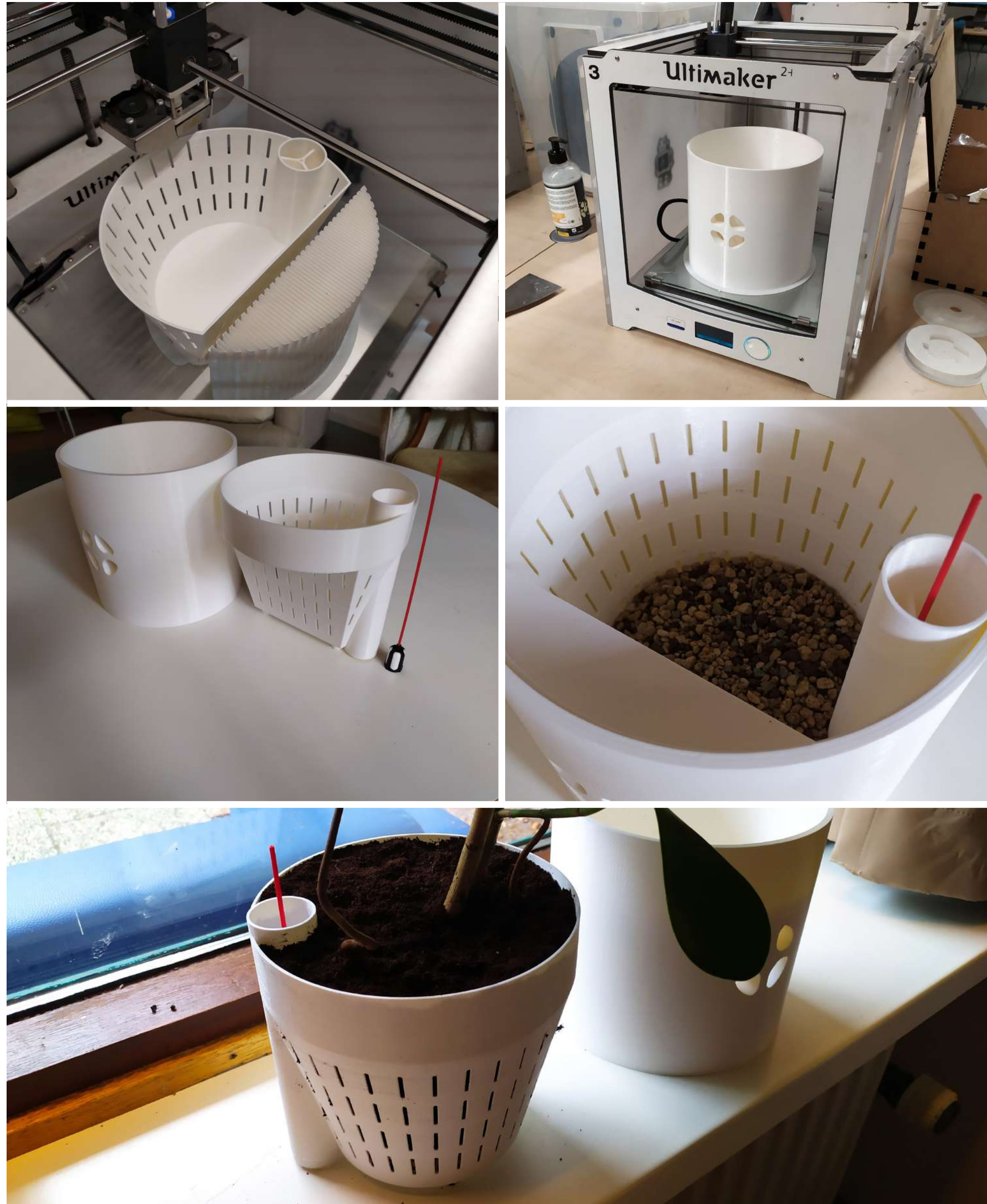
Figure 51. Prototyping of the main pot and the plant container, including the pebbles the media and the water level indicator
