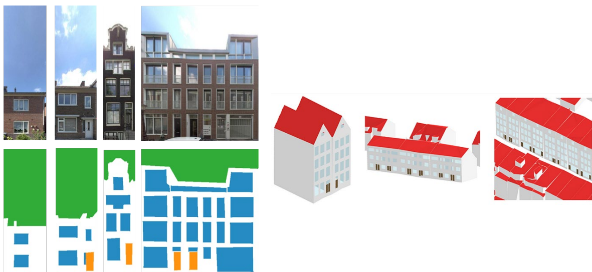
Figure 2-8 facade steps from google Streetview (top), façade masks (middle) to LoD 3.1 (Eijgenstein, 2020)
