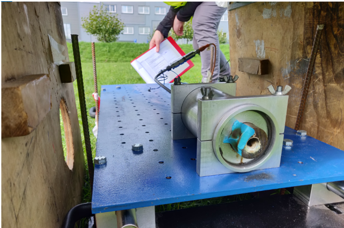
(b) BEM mounted on the test-bench with pressure sensor and igniter mounted (shown post-test of EXC-C-04). Visible are the combustion deposits on the nozzle surface.
