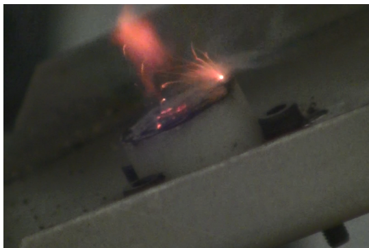
(a) Ignition of the coating (P2) showing ignition to start below the surface.
