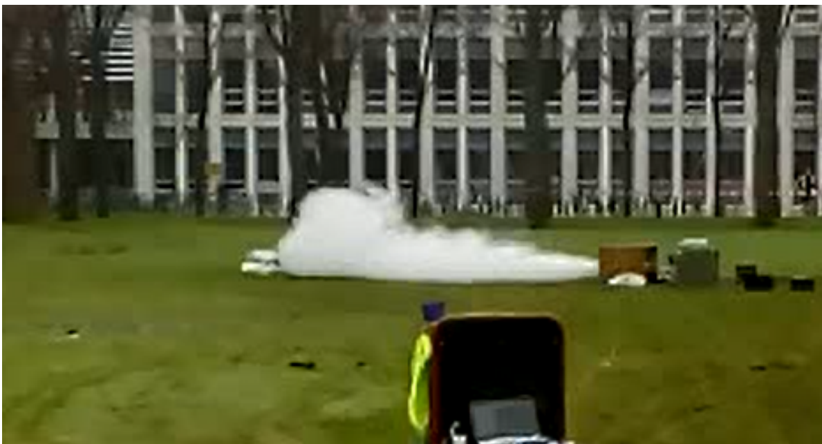
Figure E.8: Figure of an SRP test done on 21-12-2017. Shown are the shrapnel box, sandbags around the setup and downstream of the nozzle.
