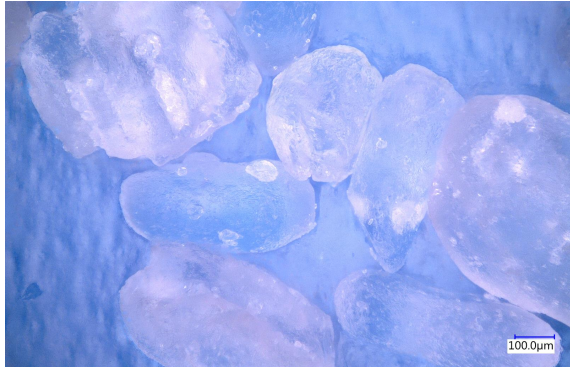
(a) Microscope image of coarse, as obtained \text{KNO}_3 .
