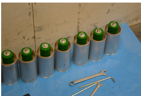
(g) Propellant cures under compression.
