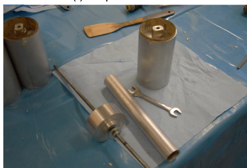
(h) Mandrel is removed.
