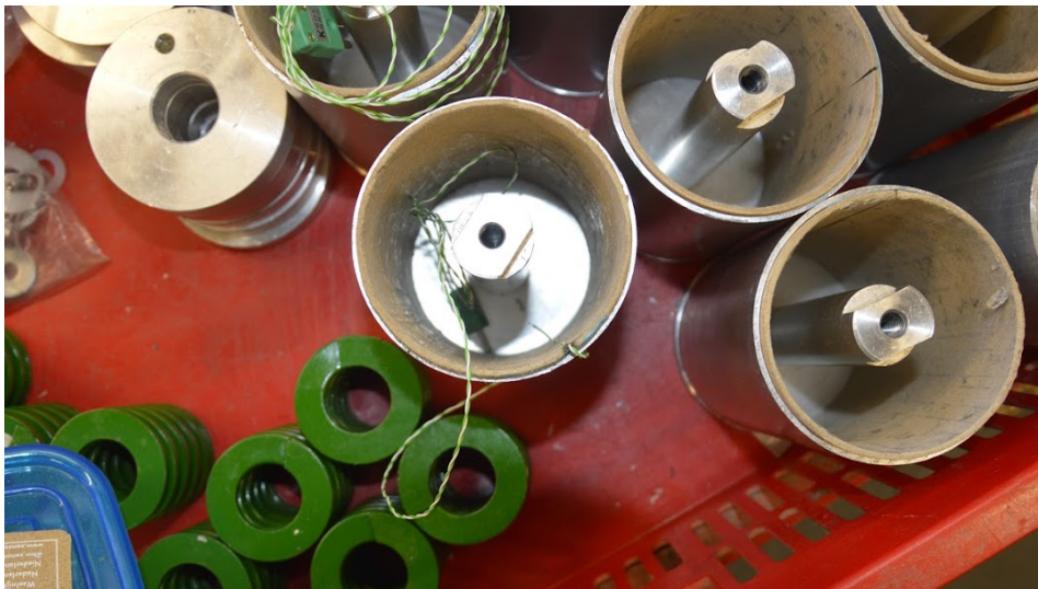
Figure 4.4: Thermocouple Placement inside the grain.
