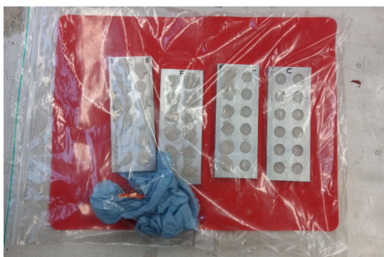
(a) Cast propellant samples in the aluminium moulds.
