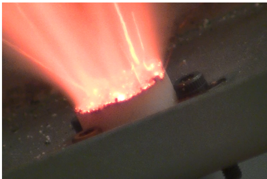
(e) Coarse Propellant flame structure showing significant active particles at the burning surface.
