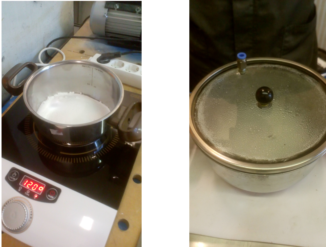
(a) The propellant samples on the induction hotplate with thermostat active. (b) The moisture condensed against the vacuum pot lid in EXA-50.
