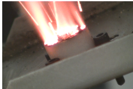
(b) Instantaneous ignition (P1) across a large part of the surface.
