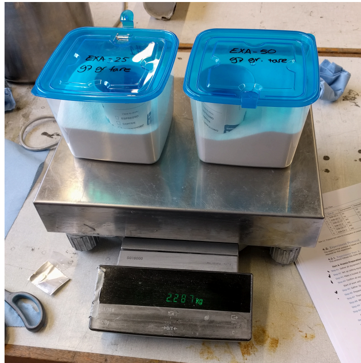
Figure 3.3: The two prepared premix batches with added moisture. Measured quantities (25g/kg and 50g/kg) of moisture were placed in the cups.
