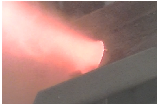
(f) Fine flame front with similar active region thinner and more evenly distributed.
