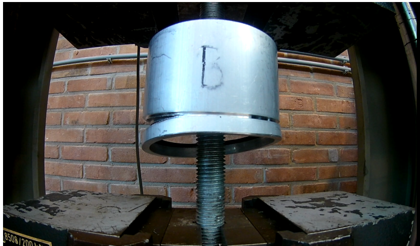
Figure E.10: One of the failed chambers inside the test setup.
