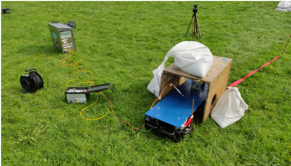
(b) Detailed view of the experiment setup with C-RIO inside the steel container, firing system (green ammunition box), test bench and sandbags. Firing direction is away from the photographer. Photo taken after firing EXC-C-04.
