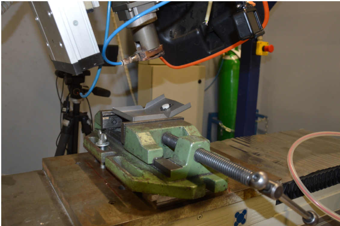
(b) Close up of sample holder (with sample) for the laser ignition experiment.
