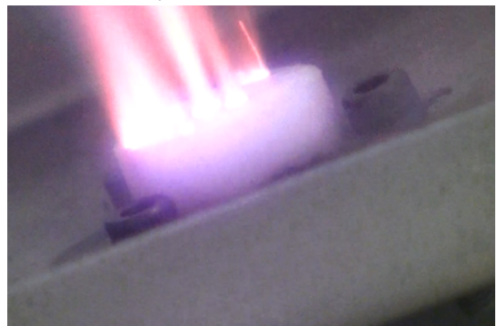
(h) Uneven ignition at very high incident flux.
