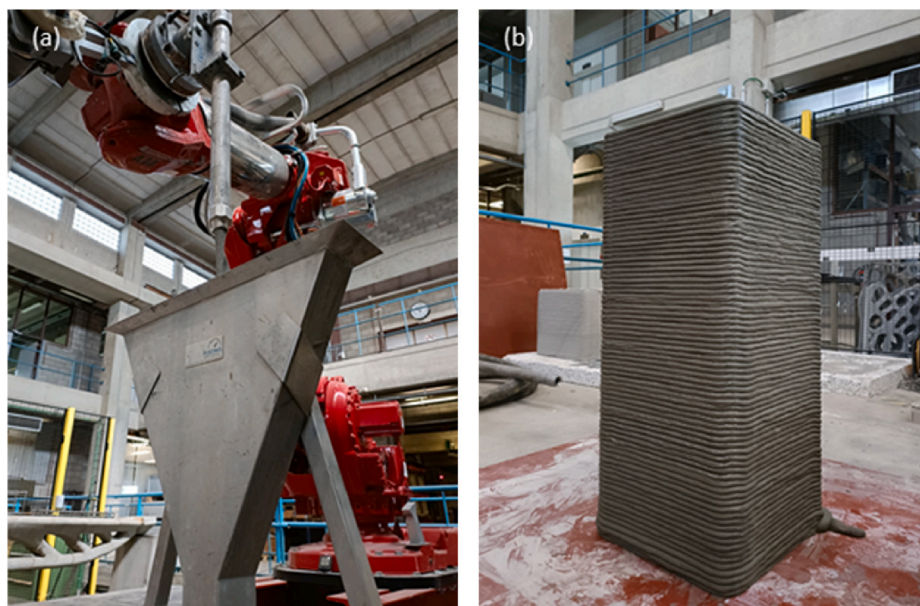
Fig. 16. Validation of the two-stream AAM concept (a) Scenario 1: Self-compacting application (with M1); (b) Scenario 2: 3D-Printing application (with M4).
