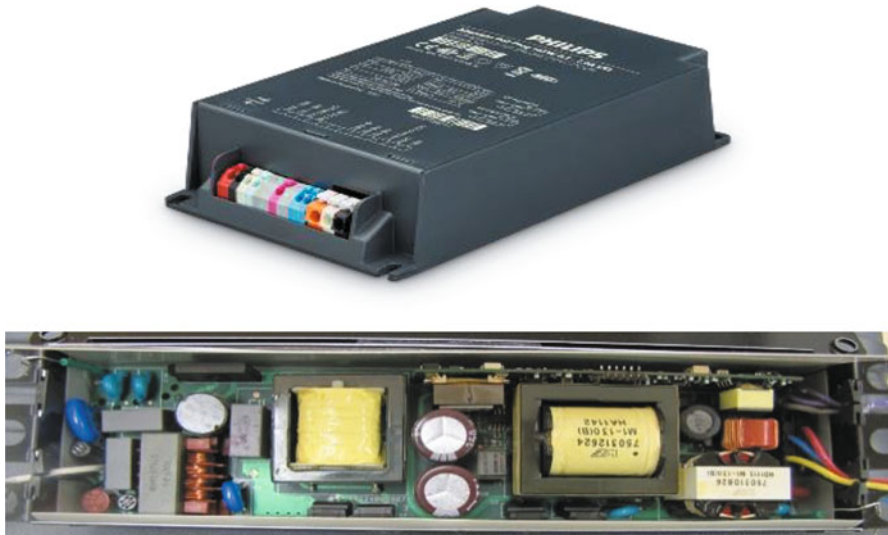
Fig. 13.1 Typical outdoor drivers used in street lighting system
