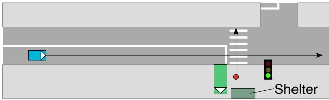
Fig. 4: Illustration of the Test Case. The AV (blue) approaches a pedestrian (red) occluded by a parked truck (green).
