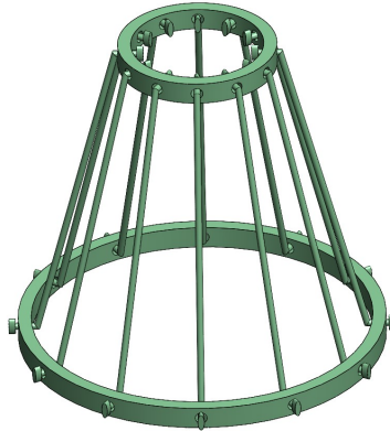
Figure 2.5: Initial metamaterial geometry (Bessa et al. [14])
