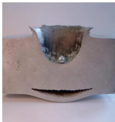
Figure 1.2: Impact of a 1.2 cm diameter aluminium sphere into an 18 cm thick aluminium block, courtesy of [7]. On the top of the target the impact crater is clearly visible, along with the ejecta baffles protruding out of its sides. On the bottom, spall fracture can be observed clearly.
