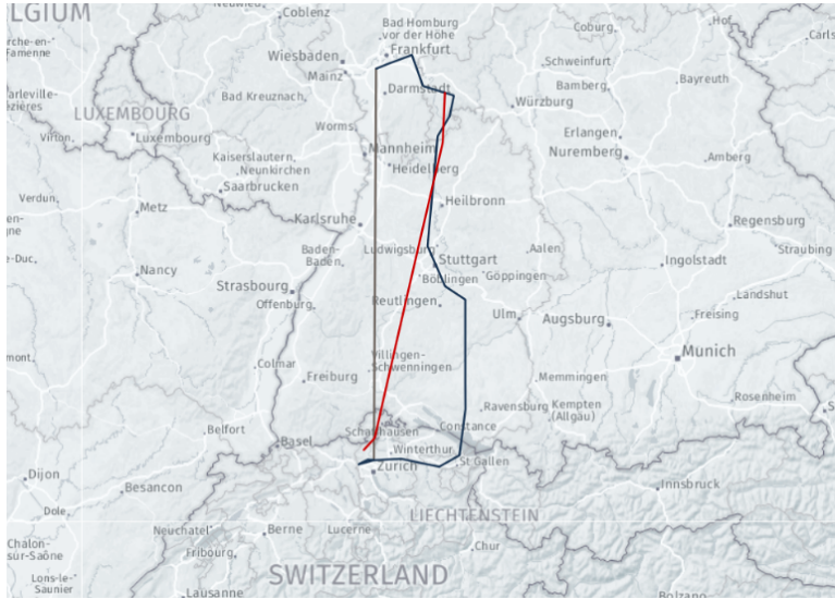
Figure 10: Trajectories of flight 2560981; Flown trajectory red, flight plan trajectory blue, great circle distance gray.
