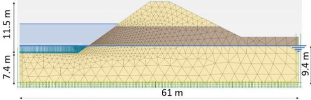
Figure 4. FEM model geometry with mesh and boundary conditions for the PlaxFlow calculation: The initial water level of the river is indicated with blue arrows and corresponds to the height of the constant head boundary condition on the right edge of the model (initially no hydraulic gradient). The variable water level is indicated in blue on the left.
