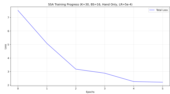
Figure 13: SSA training curves for the hand_roi_net module. Significant parameter unfreezing required, reducing batch size to 16 due to VRAM constraints.
