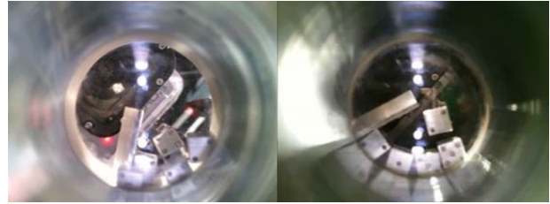
Fig. 5. Pictures taken during the 0g flight test of stacked dice(left) and a successful clamp(right)
