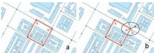
Fig. 4. (a) Water demand Q_{demand,j,w} within a mesh element w in district j , (b) Water demand at node i .
